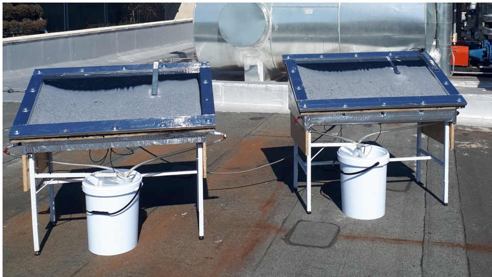
Figure A.1: A photograph from the front of two of the basin stills during operation, clearly showing the stills mounted on their frames.
