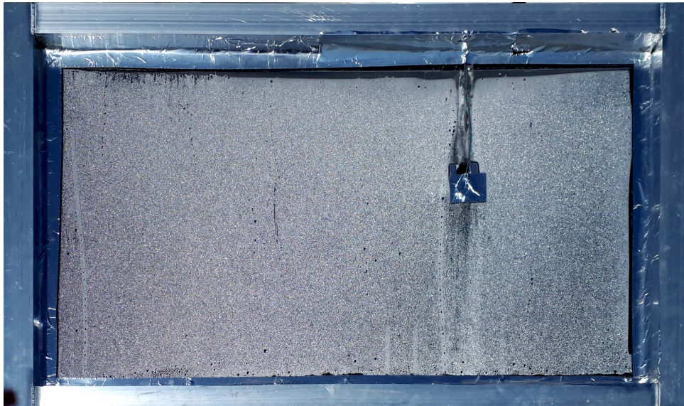
Figure A.6: A top down view of the cover plate of Still 1 on day 240, where aluminium had been added to the back wall of the still, photo taken at 10h21.
