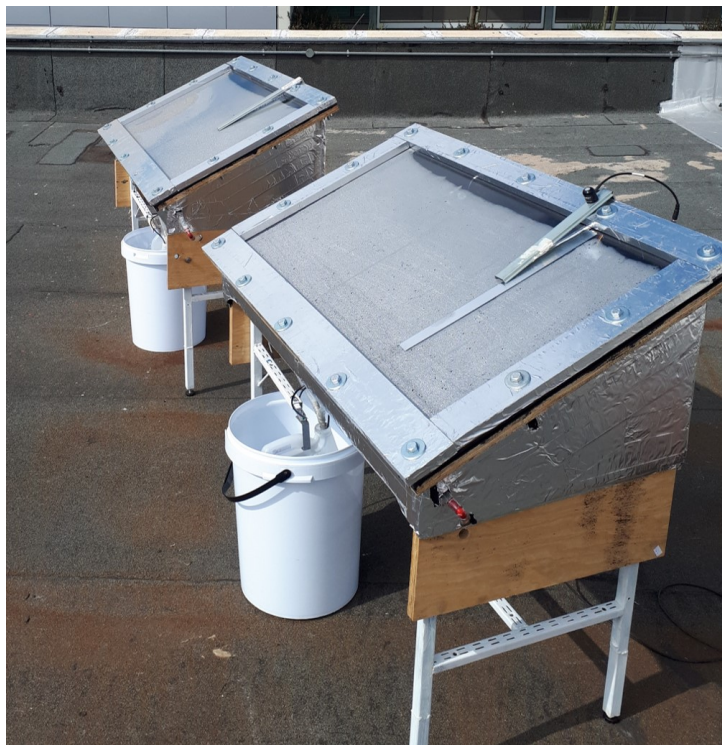
Figure A.2: A photograph of two of the basin stills during operation; the pyranometer is visible on the foremost still.
