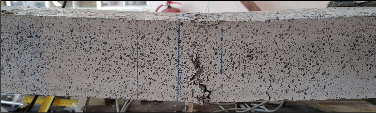
Figure B. 34: Crack formation along right span after testing
