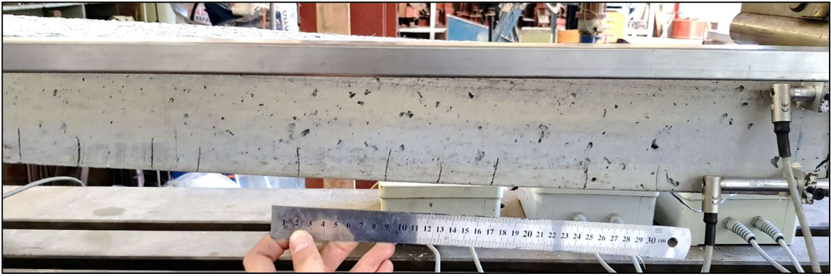
Figure B. 10: Crack spacing along right span during testing
