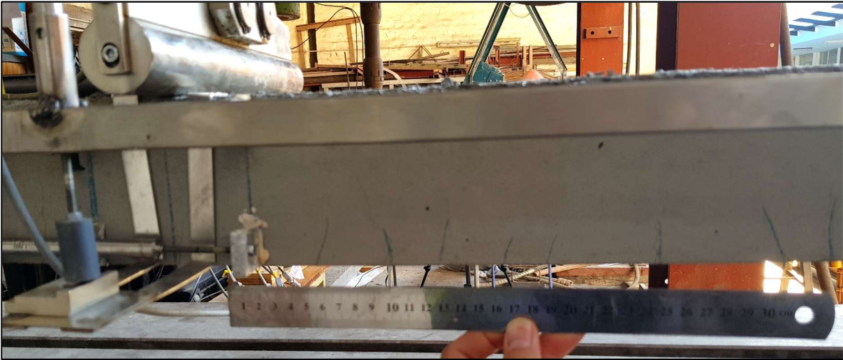
Figure B. 36: Crack formation along the left span during testing
