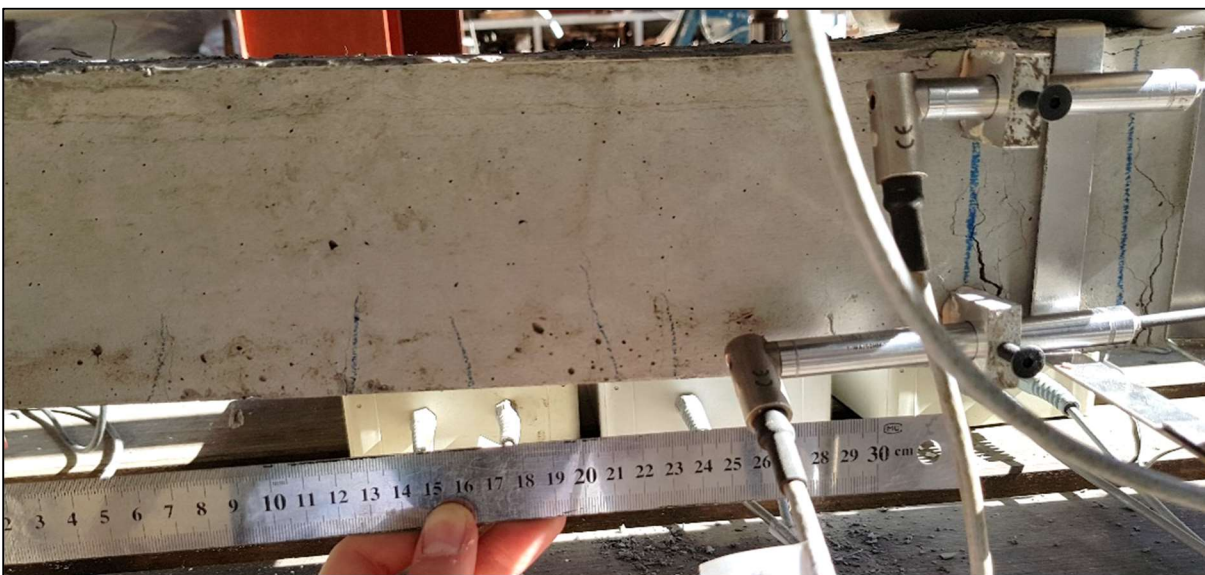
Figure B. 23: Crack spacing along right span during testing
