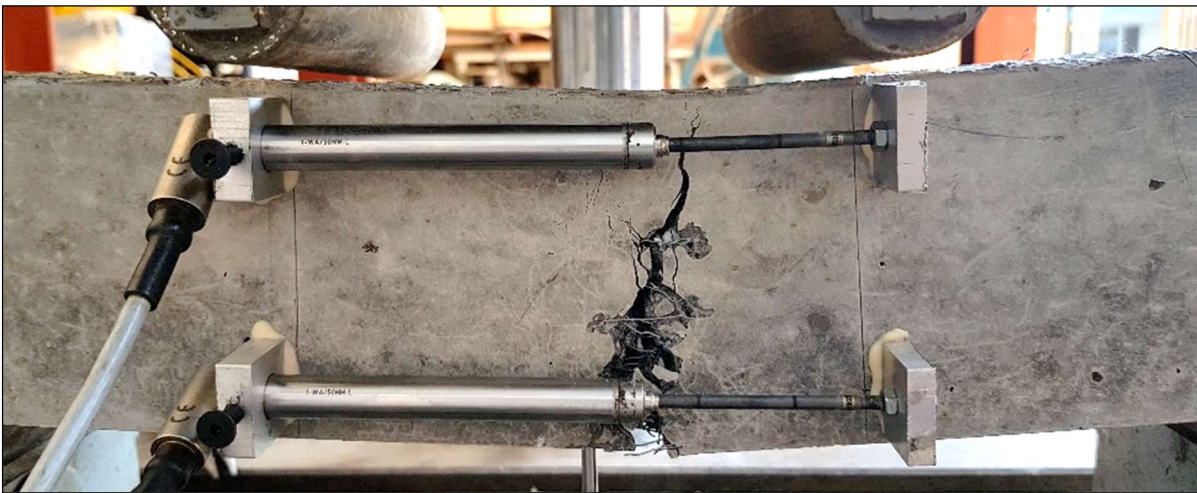
Figure 3-8: FPBT causing bending in the LVDTs
