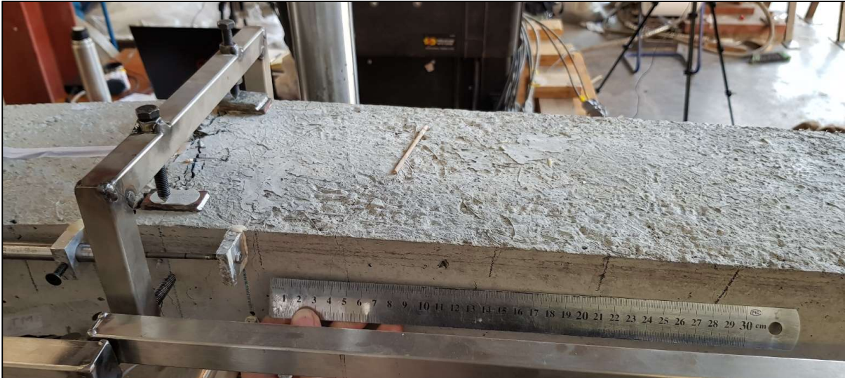
Figure B. 9: Crack spacing near centre support during testing
