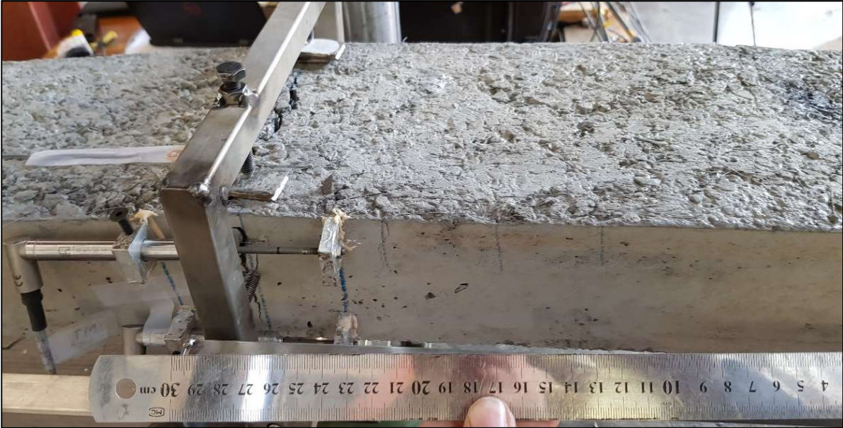
Figure B. 18: Crack formation near centre support during testing
