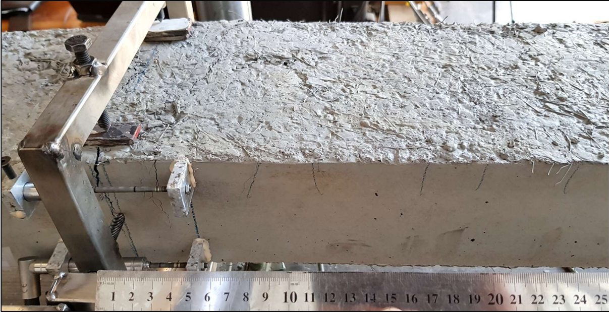
Figure B. 35: Crack formation near the centre support during testing
