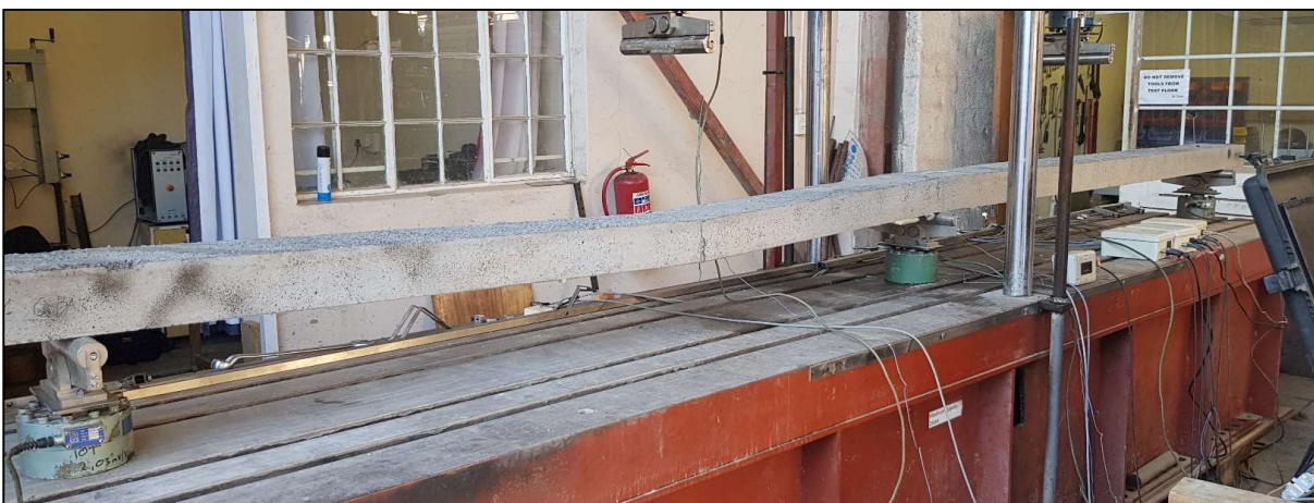
Figure B. 15: Failure at centre support and left span
