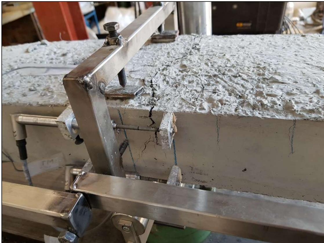
Figure B. 29: Crack formation above centre support
