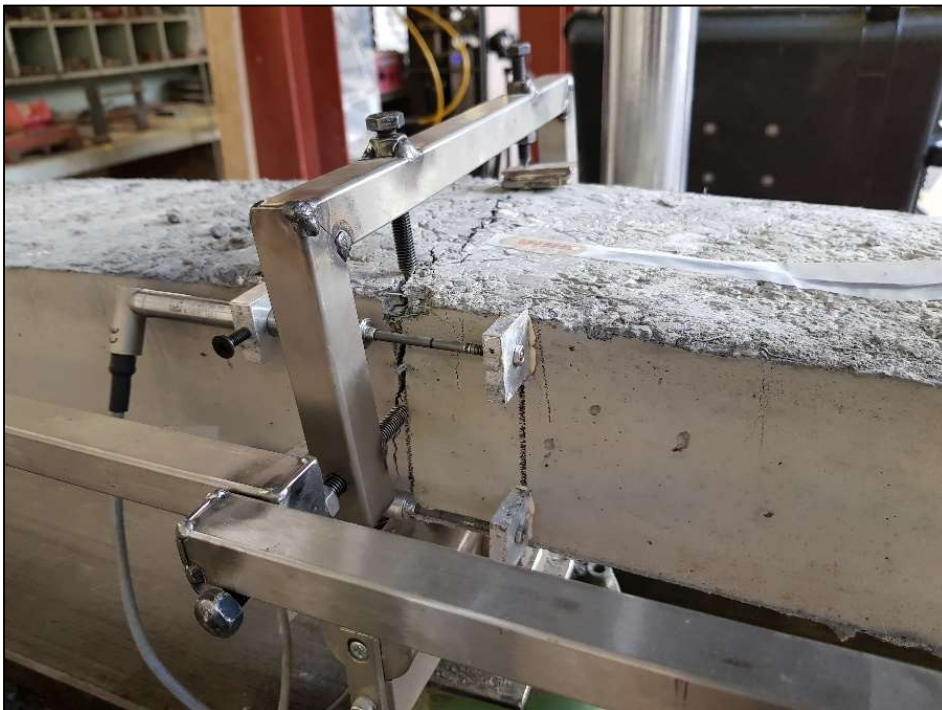
Figure B. 6: Cracking at centre support during testing
