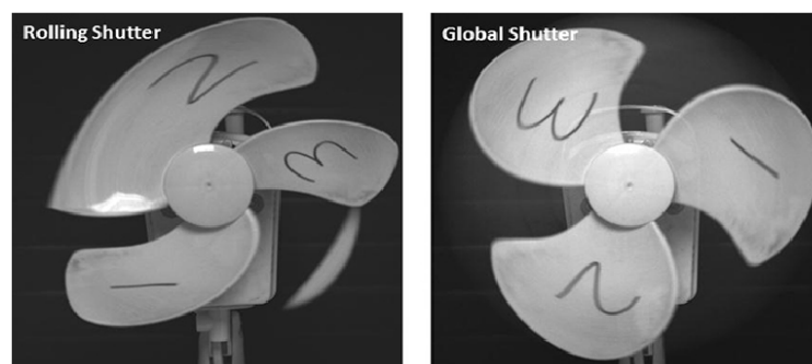
Figure 2.8. Images of moving fan blades using a Rolling Shutter vs Global Shutter (Andor, 2014)
