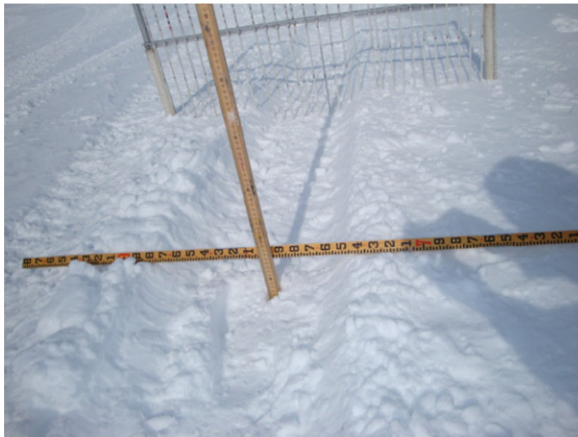
Figure 2.6. The prevailing method used for rut depth measurements (Shoop et al., 2013)
