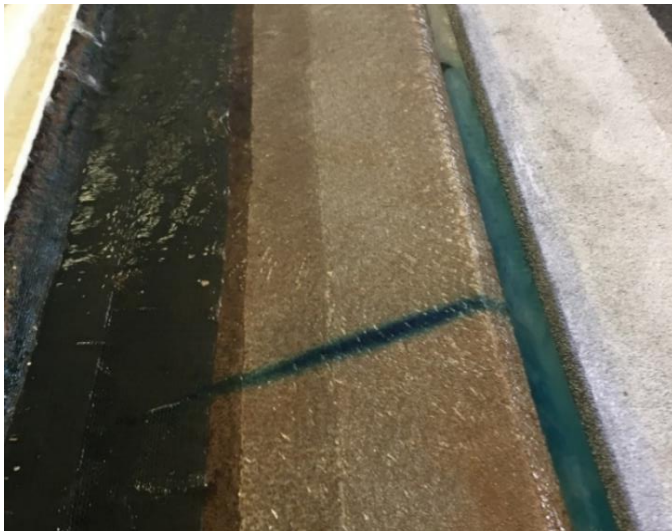
Figure 3-25: Blue dye applied to indicate water flow path slope
