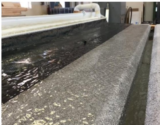
Figure 3-20: Sheet flow on the pavement model surface
