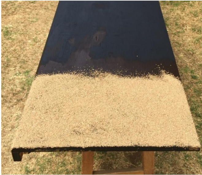
Figure 3-4: Pavement surface treatment
