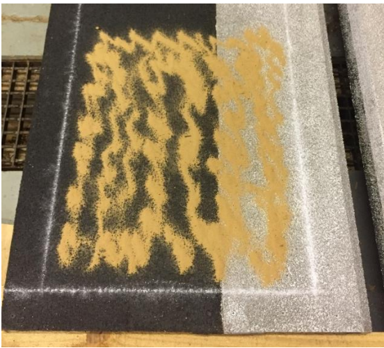
Figure 3-18: Sand spread in a zig zag pattern
