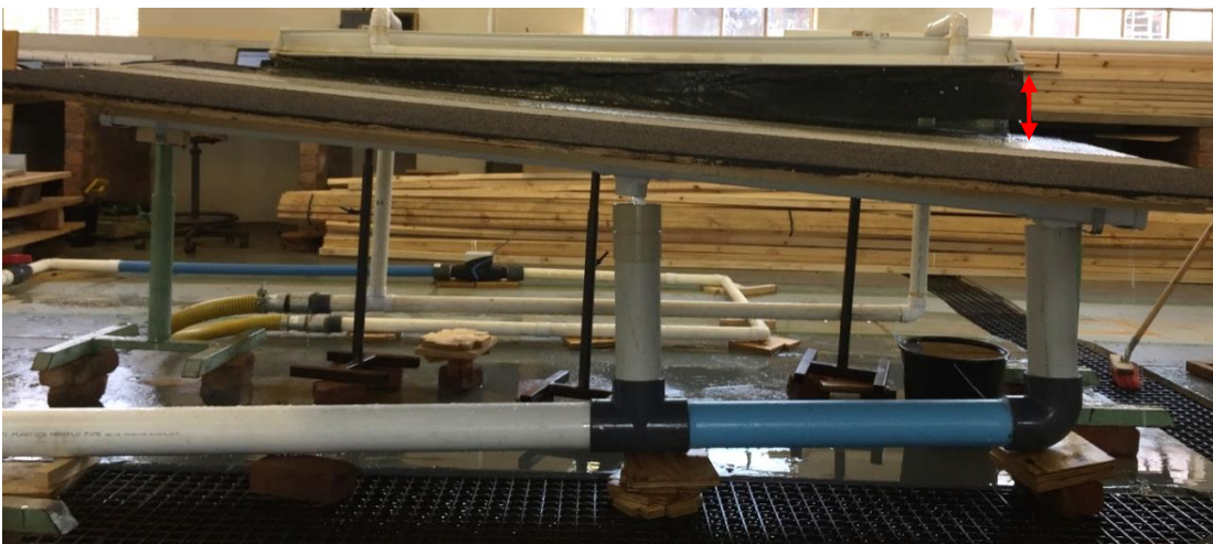
Figure 3-23: Water catchment area lifted with model slope adjustments
