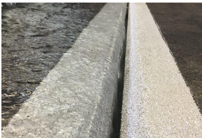
Figure 4-8: Almost 100% sheet flow interception observed for all applied sheet flow
