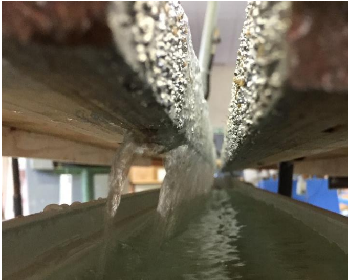
Figure 4-9: Intercepted sheet flow captured in drainage system
