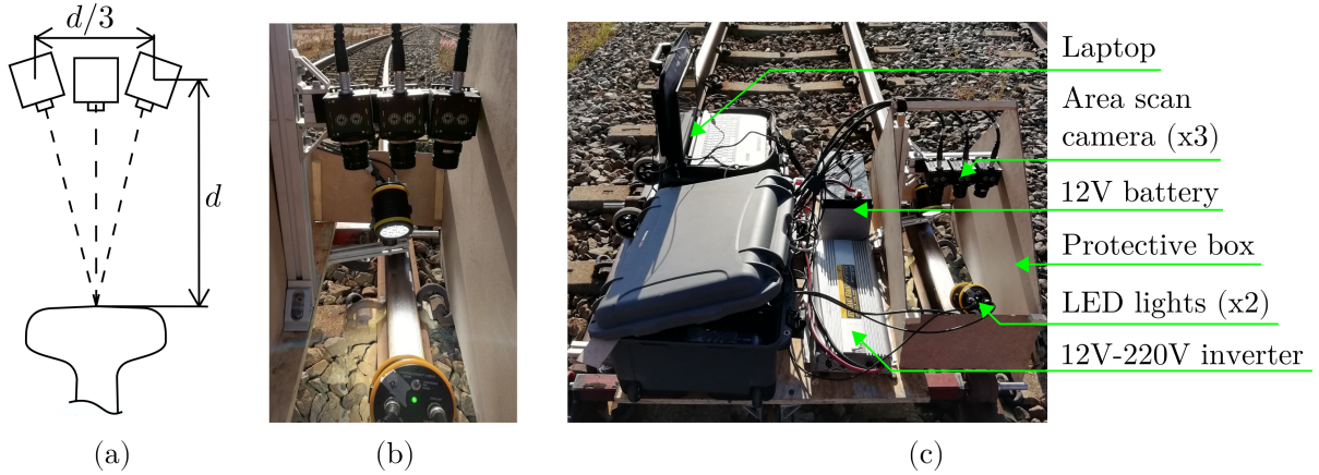
Figure 2.1: Experimental rig. (a) Schematic of camera placement. (b) Close-up of the cameras. (c) Experiment rig set-up.
