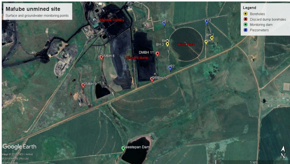
FIGURE 2.4: Map showing the boreholes (BH1 - BH4), discard dump boreholes (DMBH8 - DMBH11) and piezometer (P1 - P3) locations, as well as the monitoring dam (Beestepan Dam) surrounding the Mafube unmined site
