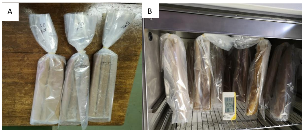
FIGURE 4.3: a) Folded bag with replicates together in one bag, b) Upright bags in a growth chamber with a temperature sensor
