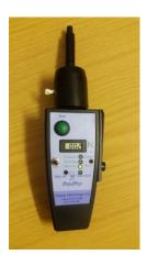
**Figure 3.1** ProdPro is a hand-held Mechanical Algometer that evaluates the mechanical nociceptive threshold (MNT) to pressure by applying steadily increasing pressure. It measures the pressure in Newton (N) ranging from 0.1 to 32 N with an accuracy of  $\pm 0.5$  N.
