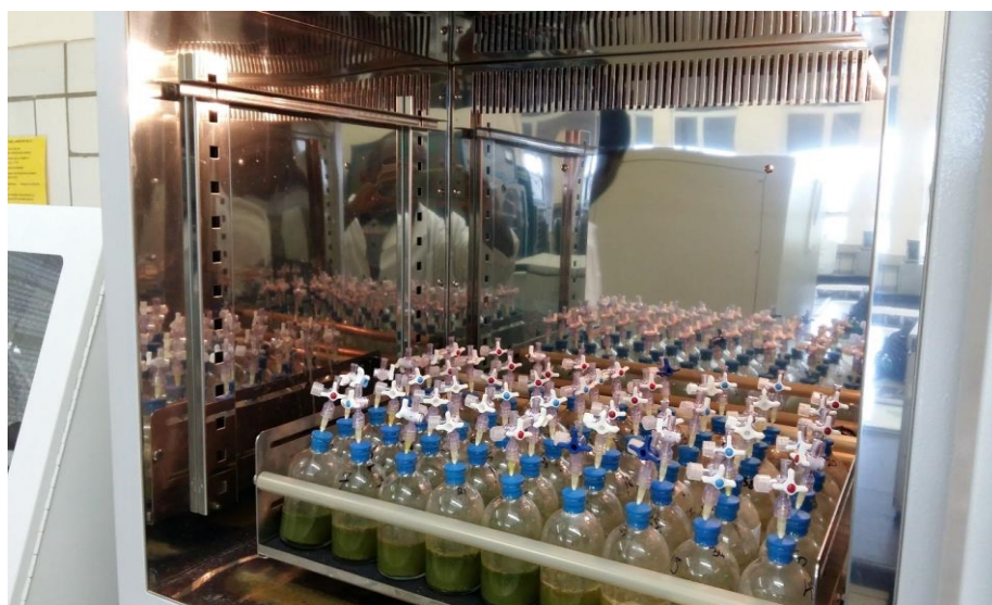
Incubating vials with modified tap with butyl stoppers
