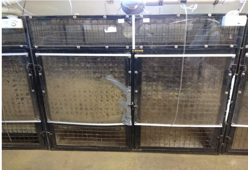
Figure 5.1a. Open-circuit respiratory chamber for small ruminants, University of Pretoria.
