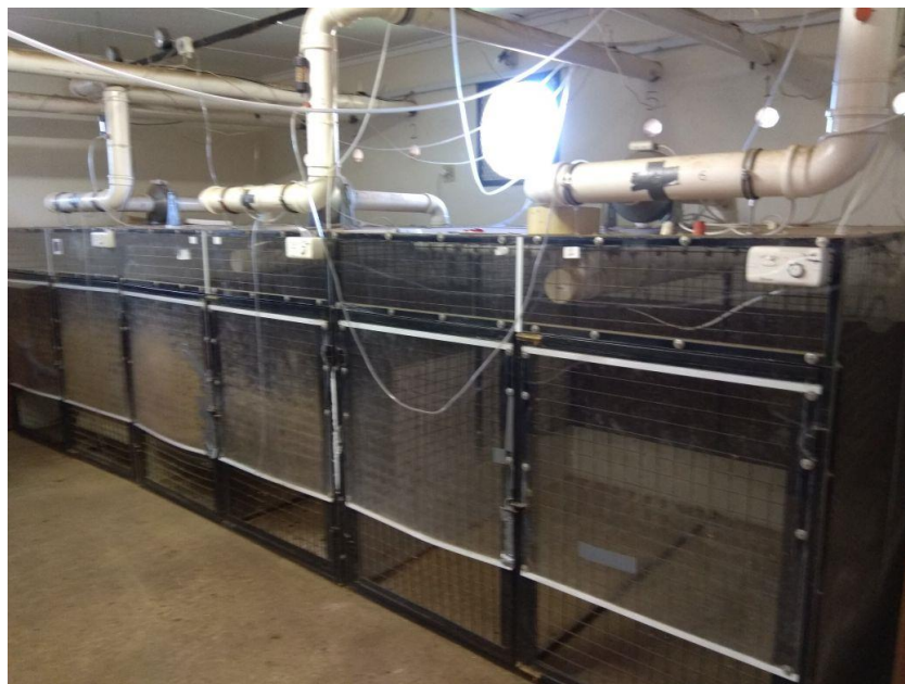
Figure 5.1b. Open-circuit respiratory chamber for small ruminants, University of Pretoria.
