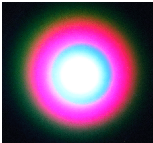
FIGURE 3.2: Optimized white-light filament generated in a 4 mm YAG crystal. The red outer circle is a remnant of the fundamental and should be cropped out using an iris.
