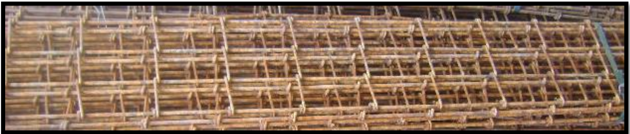
Figure 30: Osro Strap support used within underground workings (L. Meyer, 2017).
