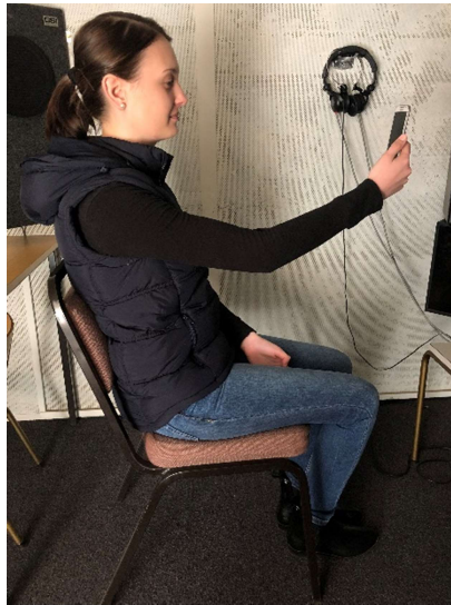
Figure 2. Position of participant and smartphone during testing with smartphone speaker
