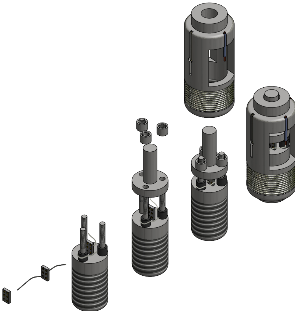
FIGURE 3.9: A demonstration of how samples are mounted into the sample holder and electrical connections are made.
