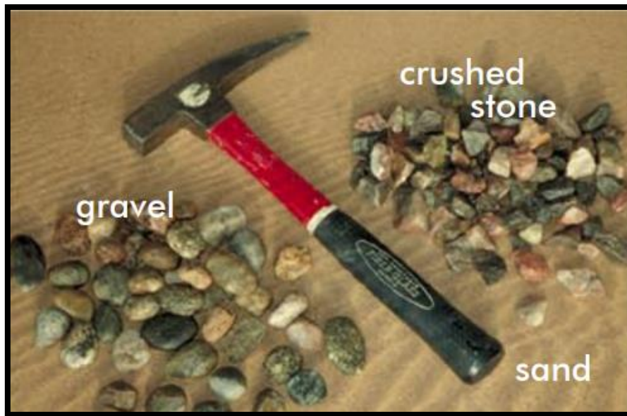
Figure 2: Illustration of the types of aggregate according to particle sizes (the hammer is for scaling purposes) sourced from (Langer, Drew, & Sachs, 2004).
