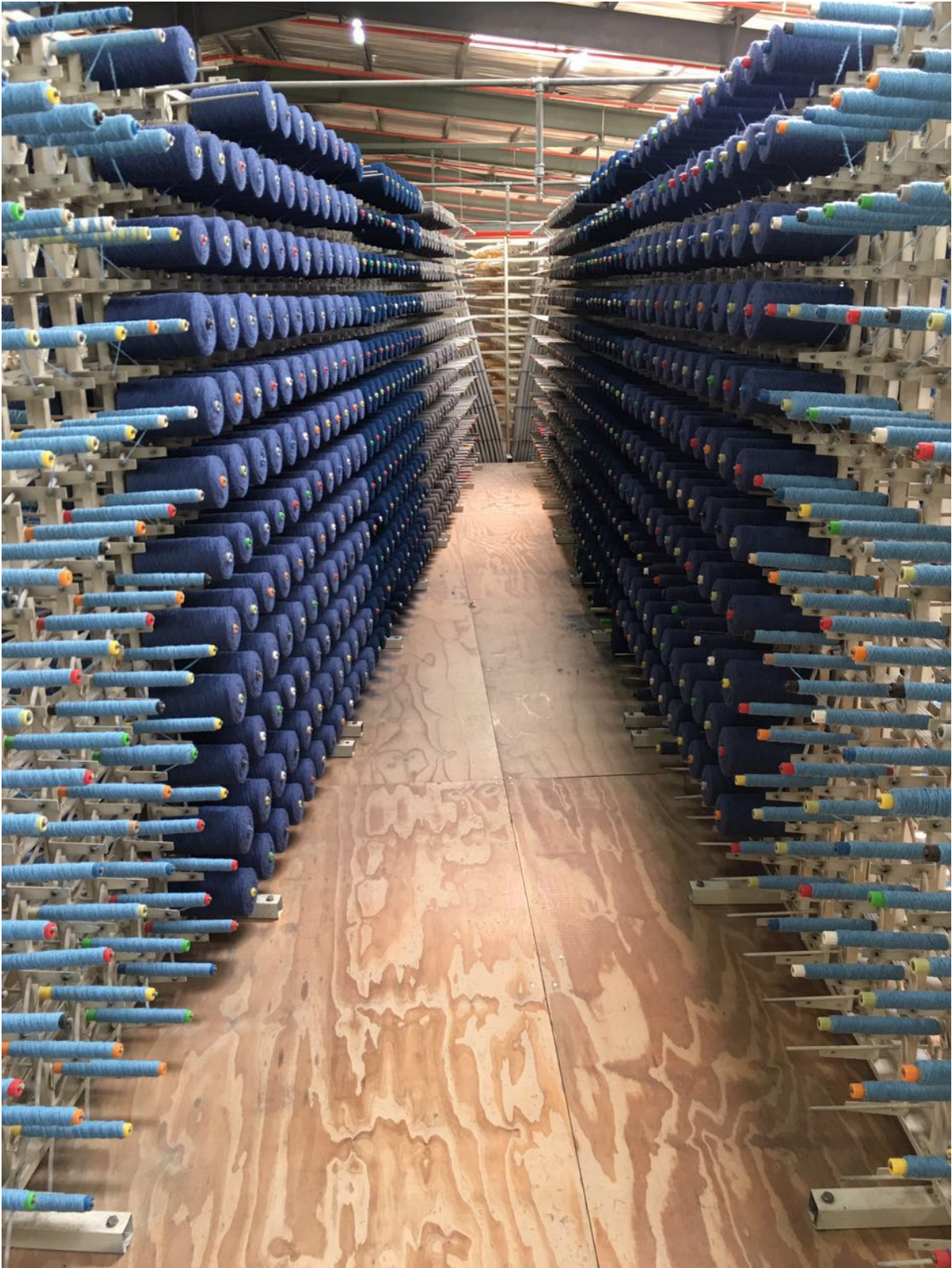
Figure B.3: Image of 1 of 8 sections of a creel on top of a loom.
