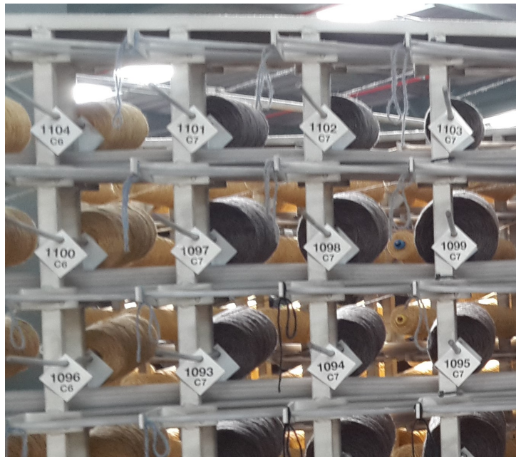
Figure 4.3: A picture showing the layout of bobbin position numbers in a creel.
