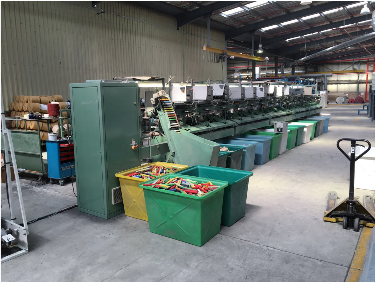
Figure B.2: Image of the winders with the bins catching the bobbins.
