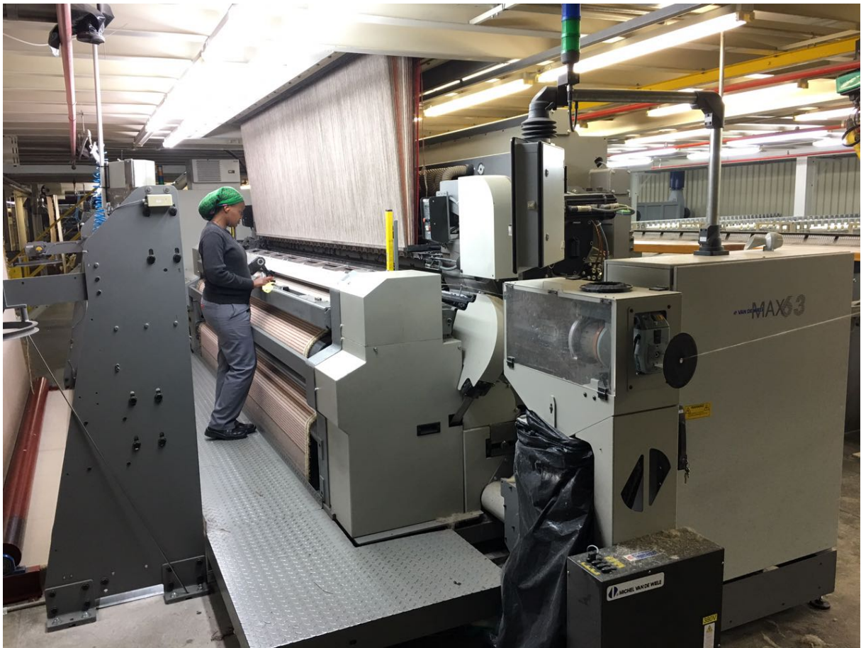
Figure B.4: Image of 1 of the 5 looms at MONN. The looms are under large frames which hold the creels above.
