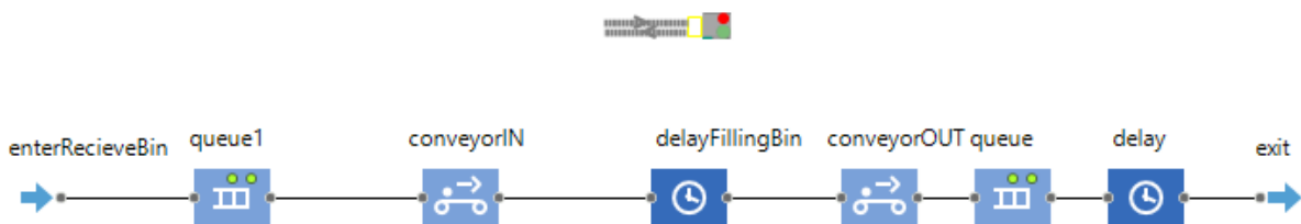
Figure 4.7: Winder with additional process blocks and conveyor units, updated WINDERMACHINE icon can be seen above.
