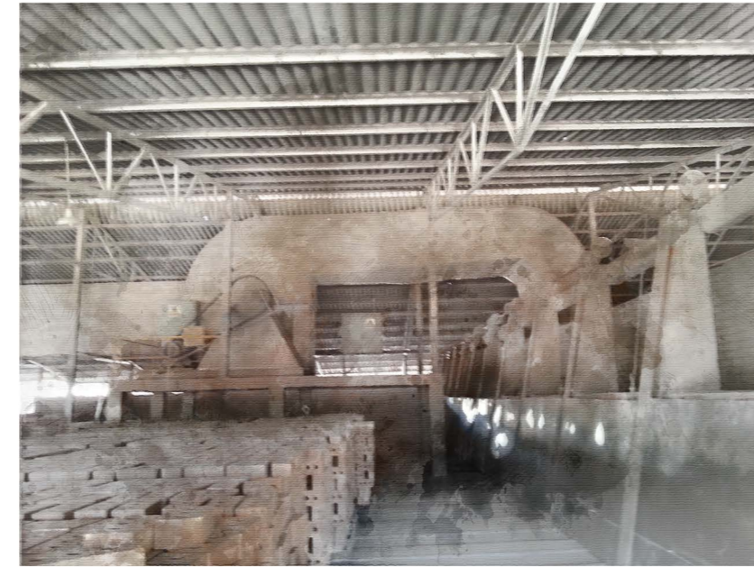
ACTIVE BRICK DRYING TRACKS
