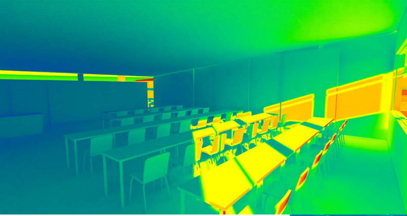
Fig 7.18 First iteration of the class room, severely over-lit and overheating. (Author 2018)
