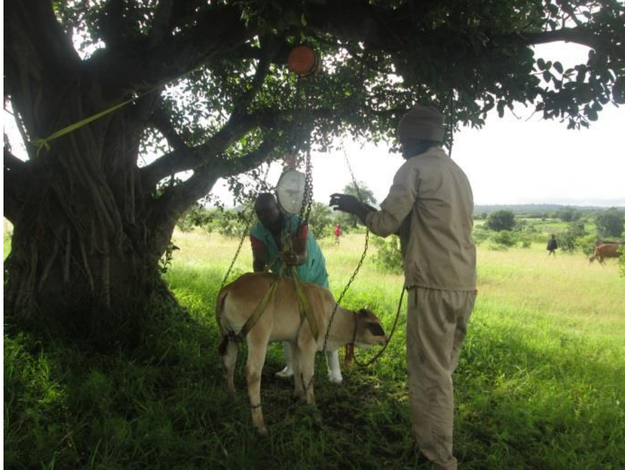
Figure 3.3: Weighing of calf using the block and tackle system and salter gauge scale
