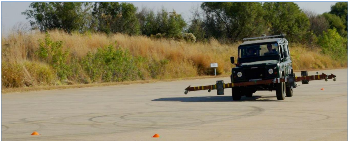
Figure 4.4: Land Rover Defender 110 Wagon doing a DLC manoeuvre in ride comfort mode
