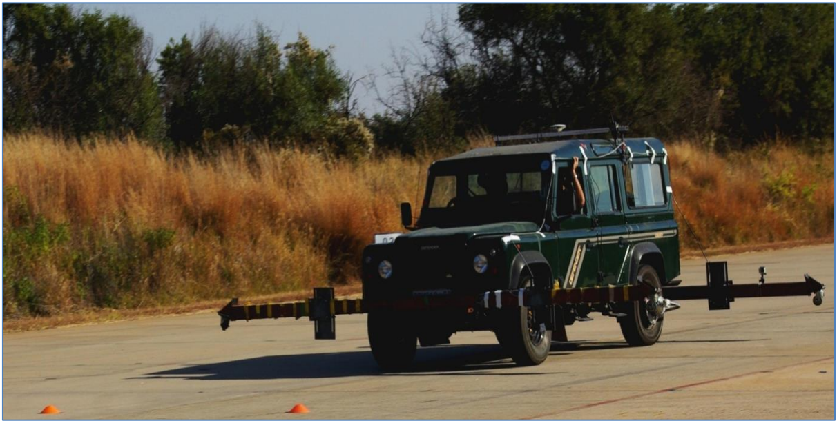
Figure 4.3: Land Rover Defender 110 Wagon doing a DLC manoeuvre in handling mode
