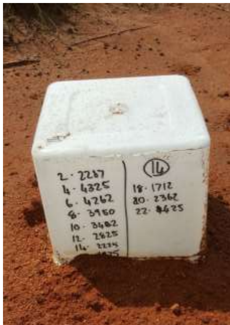
Figure 13: Plastic container covering applied beetles and dung. Ventilated at the sides with mesh (not visible in picture). Numbering on the front facing side of the container indicate penetration resistance measurements in kPa.
