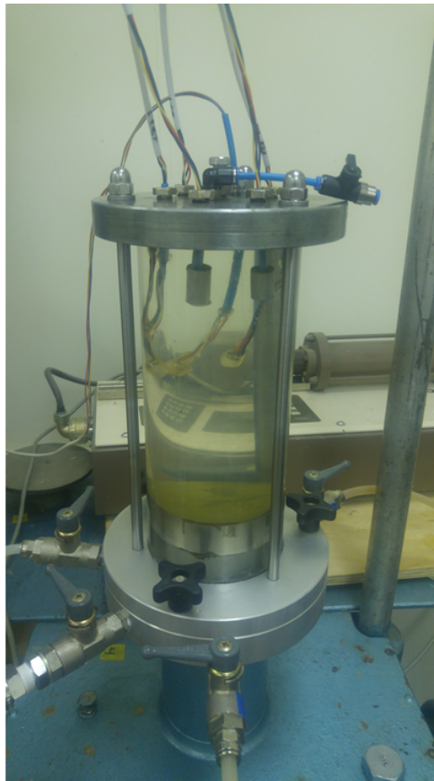
Figure 3.9: Tensiometer saturation cell during saturation
