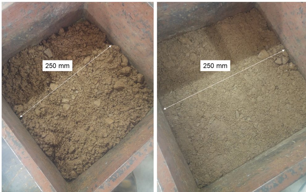
Figure 3.3: Placement of material before (left) and after (right) compaction
