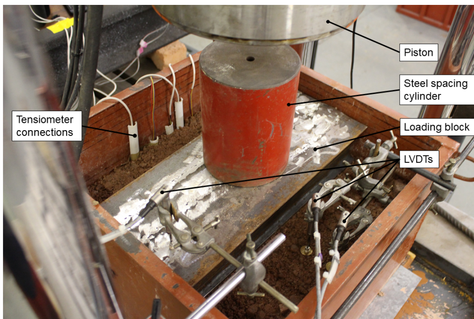
Figure 3.5: Layout of instrumentation and equipment for testing
