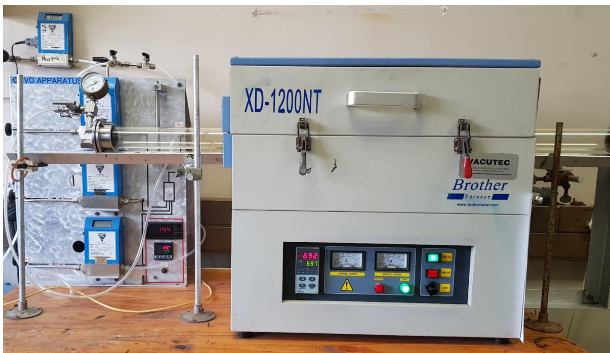
Fig.3.2: The APCVD device used for annealing in this work.
