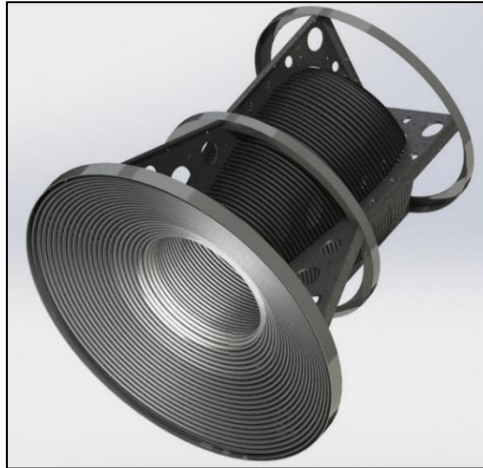
Figure 2.9: Tubular cavity receiver for direct steam generation on a dish concentrator (Pye et al., 2015)
