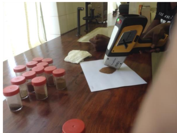
Figure 3.6: Soil samples analysed using the X-ray fluorescence technique
