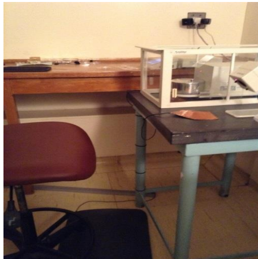
Figure 3.2: De-ioniser and anti-static mat in weighing room
