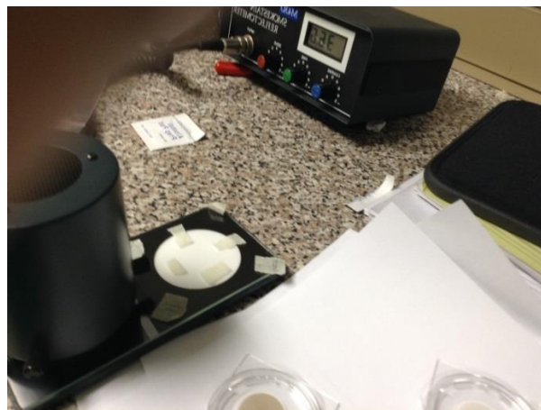
Figure 3.7: Filters being analysed for soot
