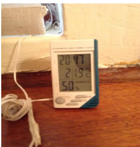
Figure 3.4: Hygrometer used to monitor temperature and humidity in weighing balance room
