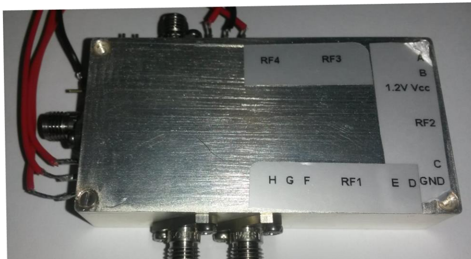
Figure 5.13. Printed circuit board enclosed in the metal casing.
