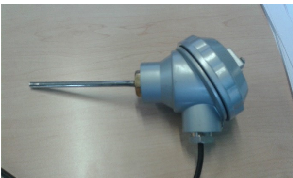
Figure 3-5: RTD 4 - 20 mA corresponding to >0 – 100 °C output
