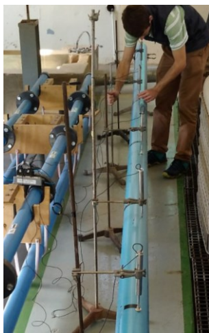
Figure B-2: LVDT setup along pipe
