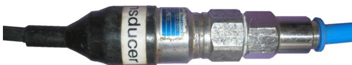
Figure 3-12: Pressure transducer (from O'Brien, 2013)
