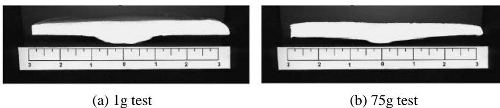
Figure 2-40: Surface depressions in (a) single gravity and (b) in a centrifuge at 75g (Dewoolkar, 2007)
