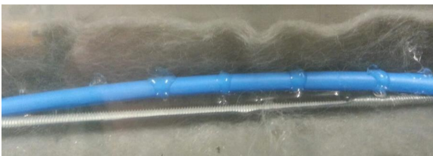
Figure 3-16: Perforated pipe on layer of Bidim, used to introduce moisture to the sample
