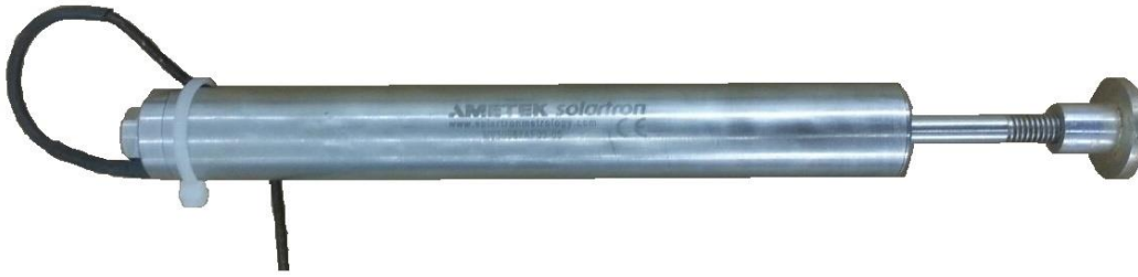
Figure 3-14: Image of Solartron Amatek S015.0 LVDT (LVDT 1)
