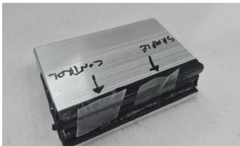
Figure 21: Film samples mounted on slabs in preparation for SEM.
