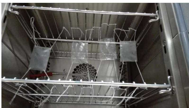
Figure 26: Setup for film oven aging tests.
