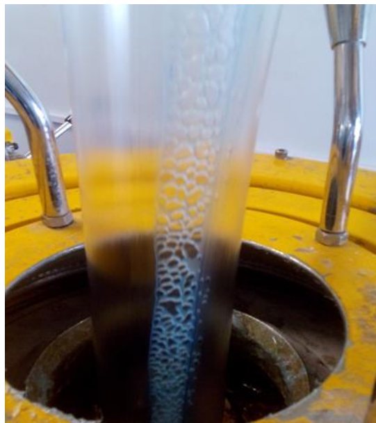
Figure 50: Trilayer film produced with bubbles due to the evaporation of malathion.
