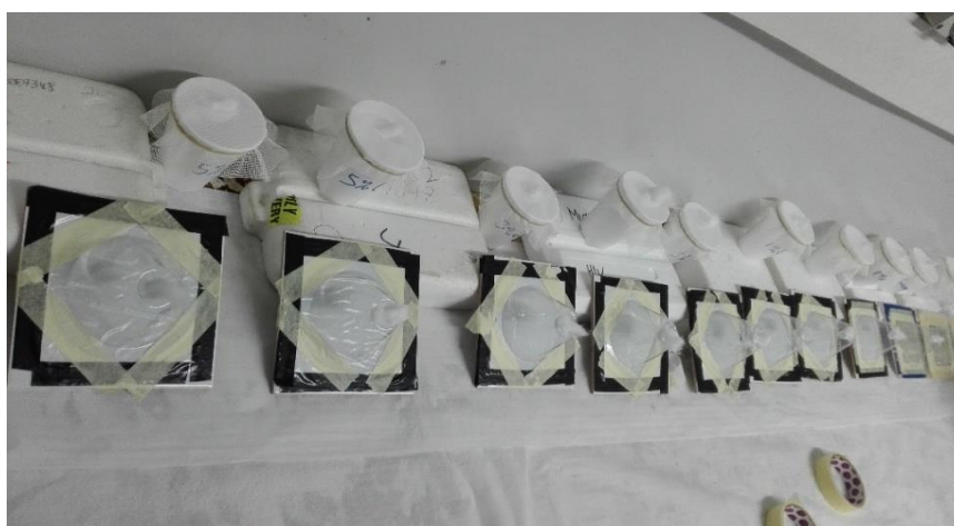
Figure 28: Setup for film cone bioassay tests.
