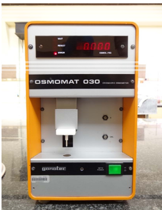
Figure 3.7: Osmomat 030, cryoscopic osmometer
