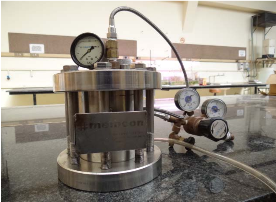
Figure 3.6: Stirred stainless steel dead-end cell
