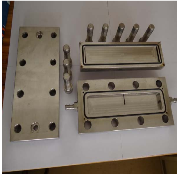
Figure 3.1: Channels of FO cell in details
