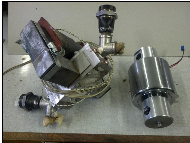
Figure 3.8: Size comparison between the MR valve by Meeser (Left) and the current prototype (Right)
