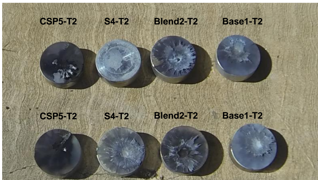
Figure 6-27: Punctured aluminium blocks after confined burn tests
