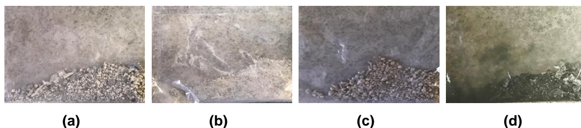
Figure 6-9: Burn residues collected after open air burn tests for (a) Base1, (b) Blend2, (c) S4 and (d) CSP5
