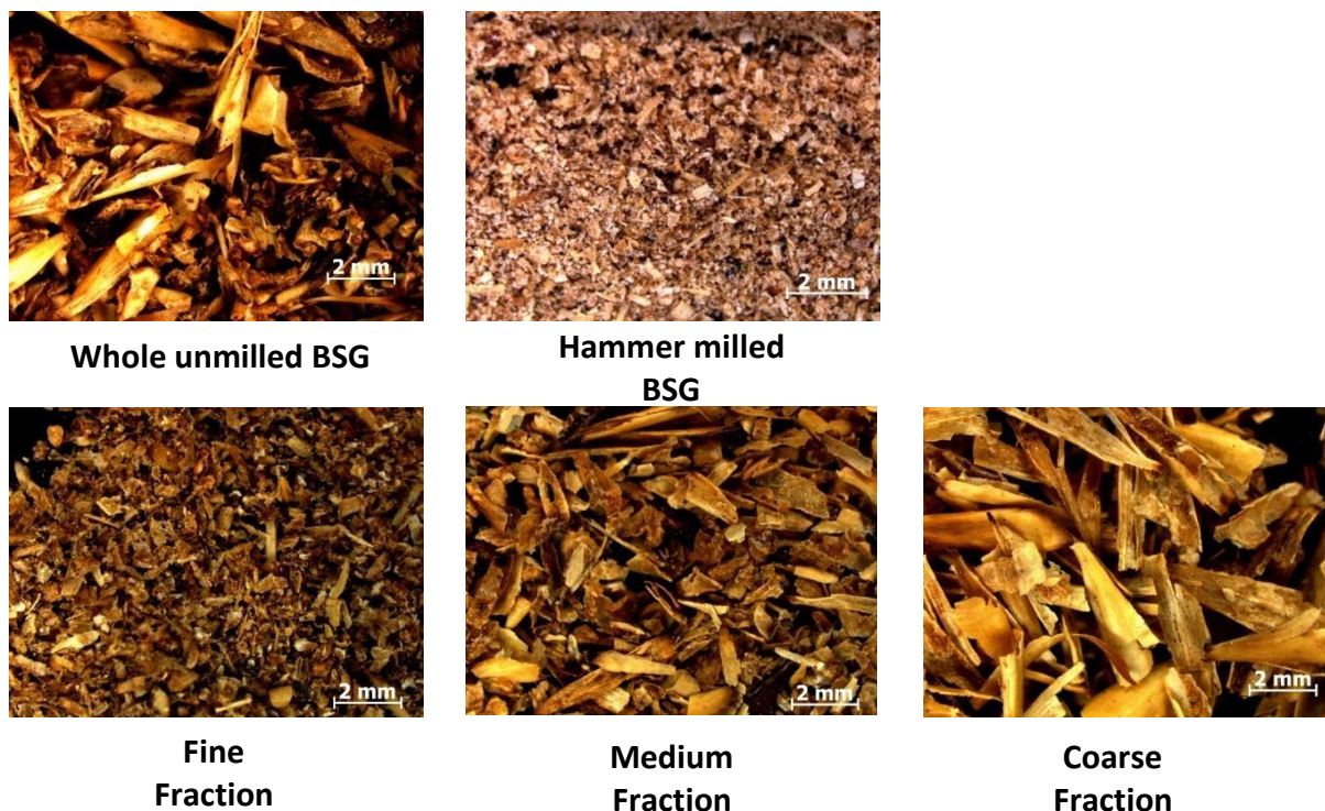
Figure 4.1.2: Appearance of the different milled BSG fractions. Fine, medium and coarse fractions are products of roller milling process.
