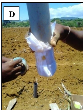
D Covering bottom of corer with nylon cloth
