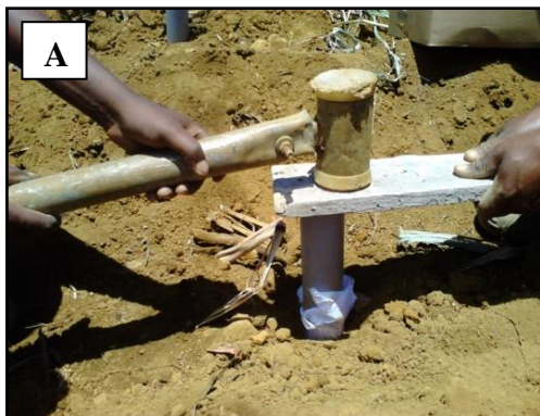
A Insertion of Polyvinyl Chloride corer 0.20 m into soil
