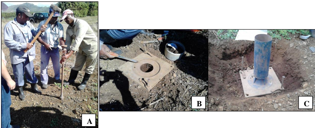
FIG.2.1.2: The corer method for the measurement of bulk density (A) and the sand tower method for the measurement of bulk density in rocky soils (B and C)
