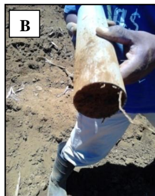
B Removal of intact soil core
