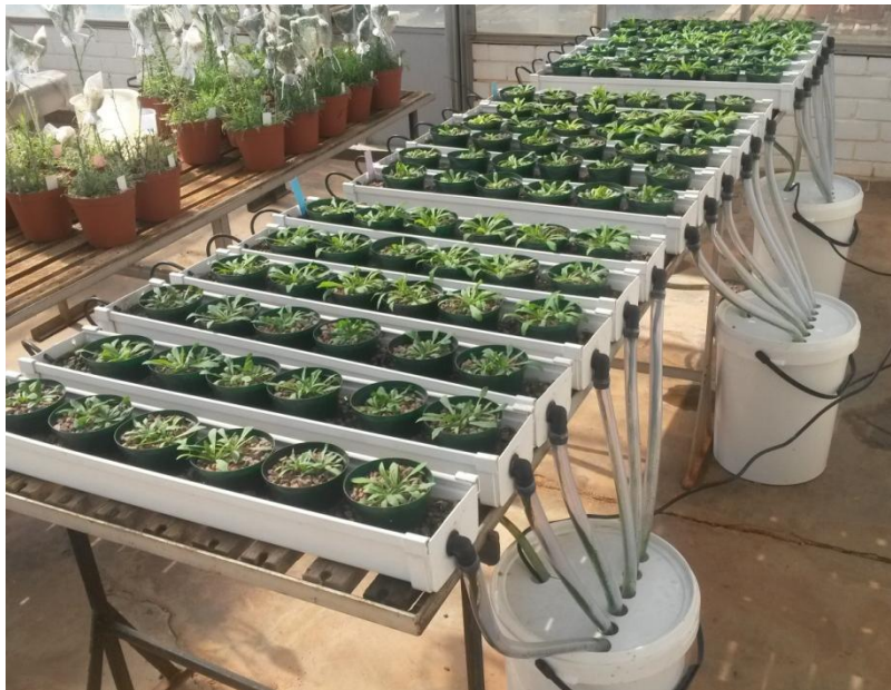
Figure 2.5 Hydroponic system for testing the response of Conyza bonariensis seedlings to glyphosate when grown in medium containing different manganese concentrations.
