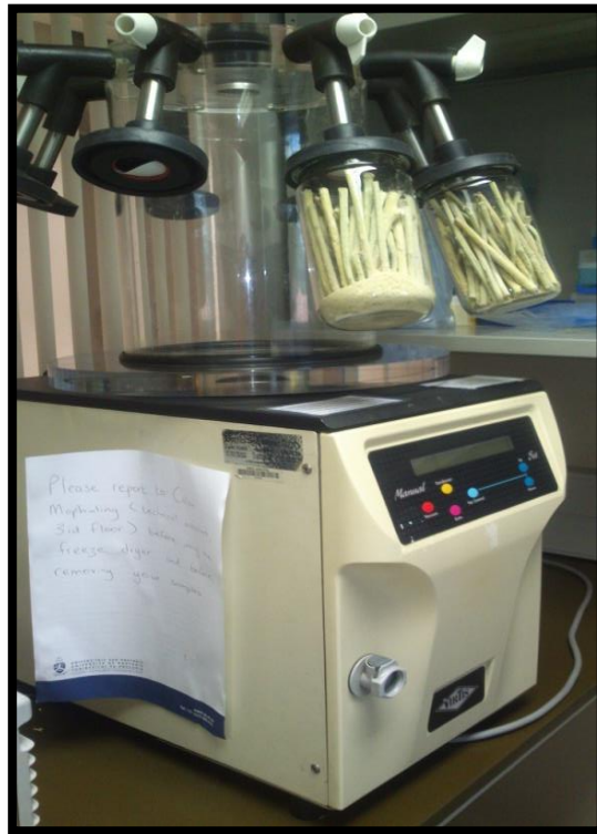
Figure 2.4: Virtis freeze drier (United Scientific (Pty) Ltd) with flasks filled with E. damarana stems.
