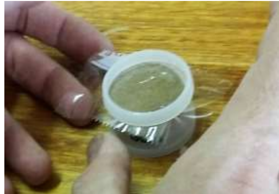
Figure 3.2.10 Placing piece of Mylar film over sample cup (left). Placing polyethylene ring on top of Mylar film and securing film in place by pressing down on polyethylene ring (right).
