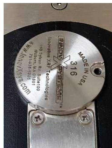
Figure 3.2.9 Mylar film roll and polyethylene sample cup (left). Stainless steel calibration coin in workstation's test chamber (right).
