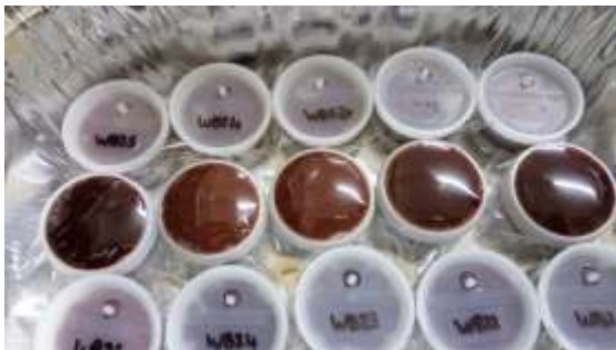
Figure 3.2.11 Finished sample cups after Mylar film has been secured and sample cups marked (left). Sample cup in inverted position in test chamber of Olympus workstation (right).
