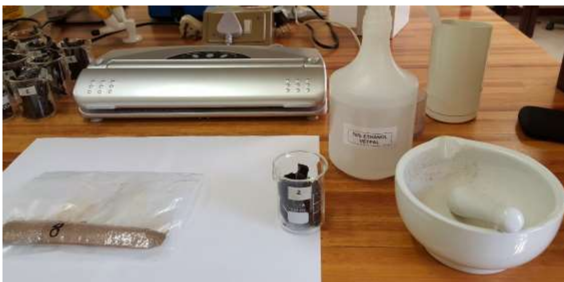
Figure 3.2.3 Vacuum sealed homogenous powder (left) with vacuum sealer in background. Ethanol spray and mortar and pestle to the right of photo.
