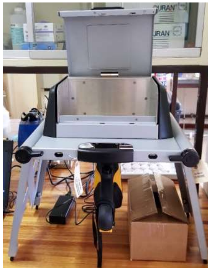
Figure 3.2.7 Olympus Delta XRF unit attached in an inverted position to the workstation with sample chamber.
