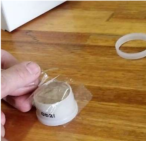
Figure 3.2.10 Placing piece of Mylar film over sample cup (left). Placing polyethylene ring on top of Mylar film and securing film in place by pressing down on polyethylene ring (right).
