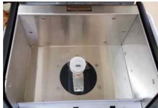
Figure 3.2.11 Finished sample cups after Mylar film has been secured and sample cups marked (left). Sample cup in inverted position in test chamber of Olympus workstation (right).
