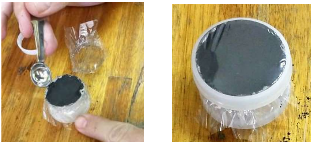
Figure 3.2.13 Dry ashed sample placed onto bottom piece of Mylar film to prevent sample from falling into sample cup (left). A second piece of Mylar film placed over sample to form an envelope (right).
