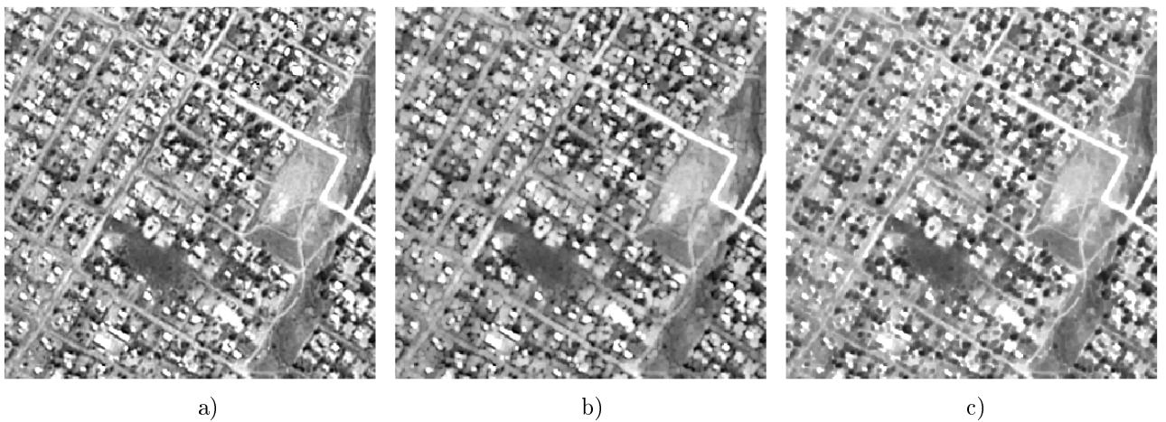
Figure 15: Opening and closing of greyscale image: a) Original image b) Grey tone opening c) Grey tone closing
