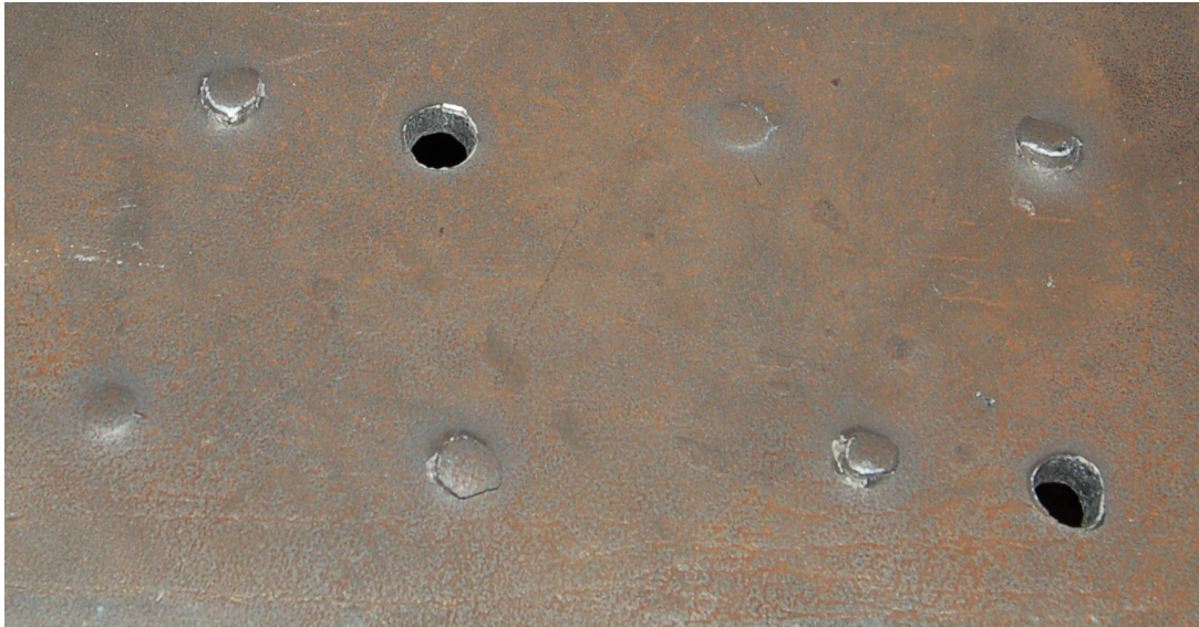
Figure 2.5: Typical plugging failure
