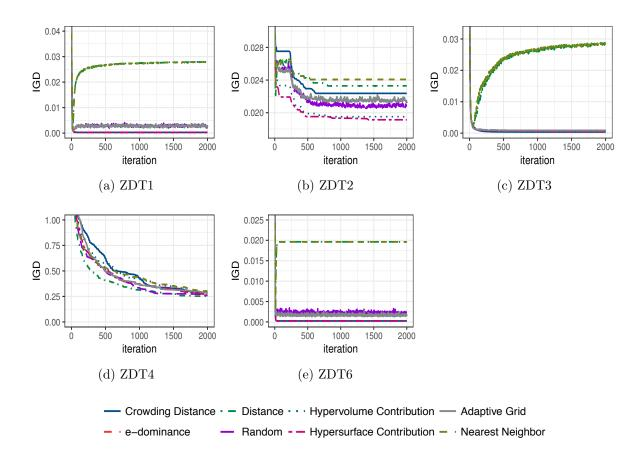
Figure 4.29: VEPSO (PCXA) Inverted Generational Distance for ZDT1 through ZDT6
