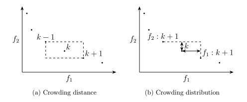
Figure 4.13: Crowding distance and distribution calculation hypercubes
