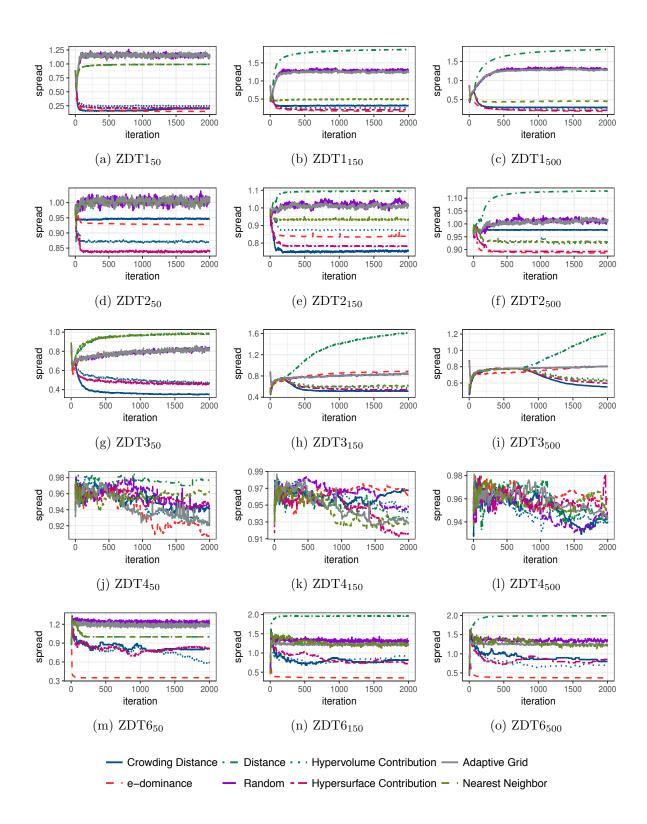
Figure 4.3: VEPSO (PCXA) spread,  $\Delta$ , over archive sizes 50, 150 and 500 for ZDT1 through ZDT6
