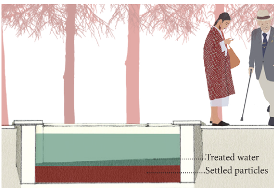
Figure 3.4 Settling pond (Author 2017)
