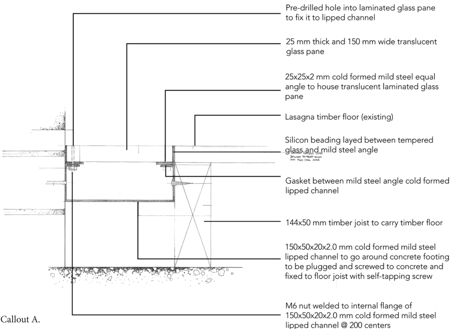
Figure 7.36 Gallery balustrade detail Figure (Author 2017) Figure 7.37 Below; Callout A, Lipped Figure channel lighting detail (Author 2017)
