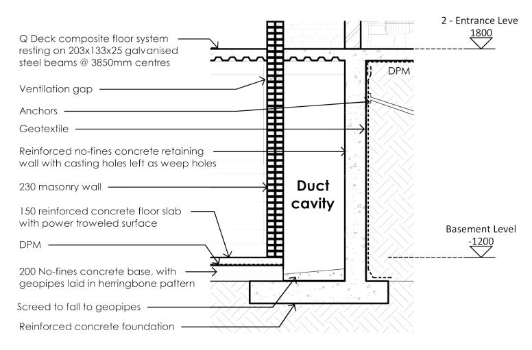
DETAIL SECTION B1 - RETAINING WALL DUCT
