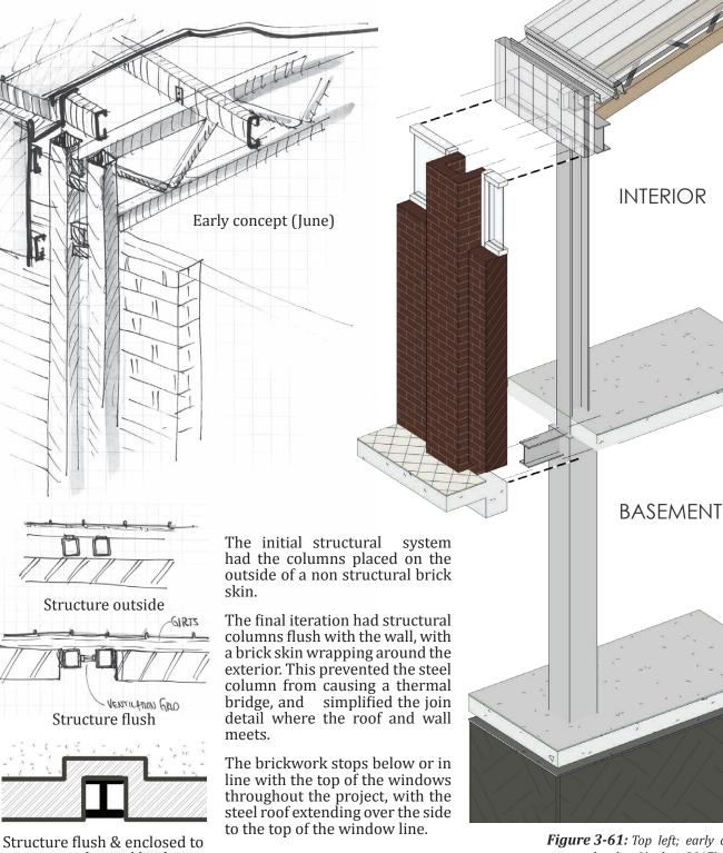
Structure flush & enclosed to prevent thermal bridge *Figure 3-61:* Top left; early construction system sketches (Author, 2017)
