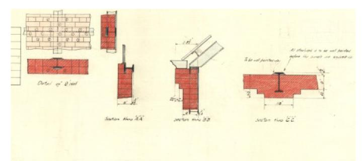
Figure 121 Steel and concrete junctions of Retort No. 1 (Lauferts le Roux & Mayunganidze 2016: 21) © University of Pretoria
