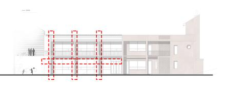
Iteration two entailed the implementation of solid infill panels in between the first floor slab and the horizontal louvres proposed in iteration 1.
