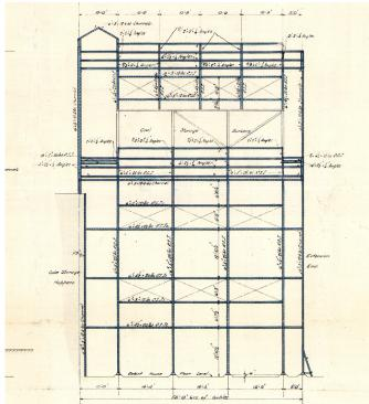
Figure 118 Steel structure of Retort No. 1
