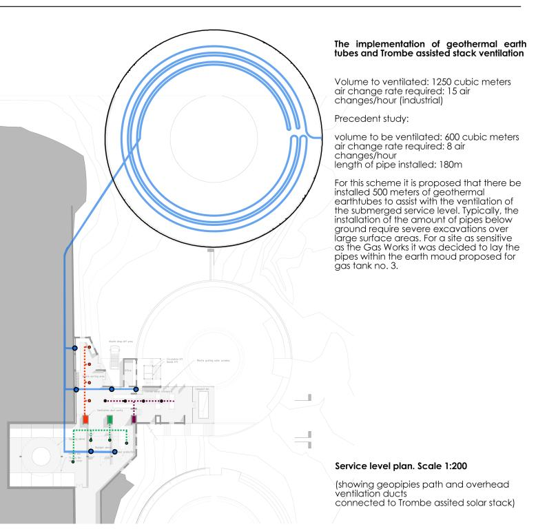
Figure 140 The implementation of geothermal earth-tubes (Author, 2017) © University of Pretoria
