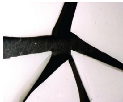
Figure 8: Light microscope picture of a fractured Cercon disc.
