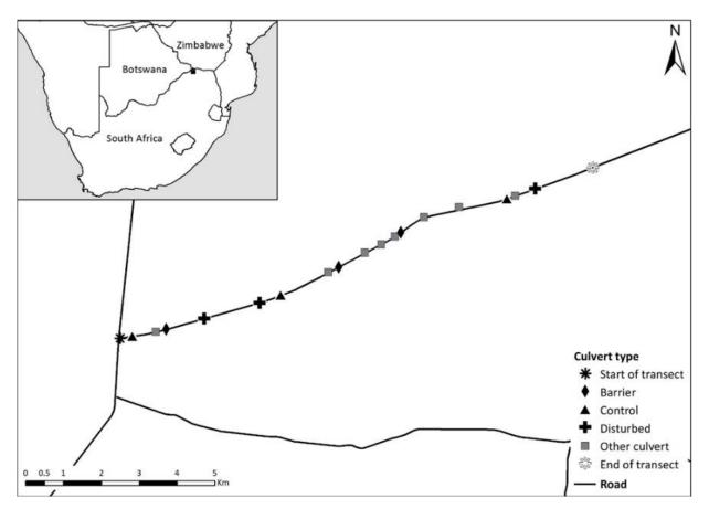
**Figure 1.** A schematic diagram showing transect start and finish and the location of the 17 culverts along the 12.3 km section on the D2662 paved road. Each culvert has been coded to show the treatment applied (barrier, control, disturbed or other (i.e. not used in the study)). Inset map shows location of study (black square).
