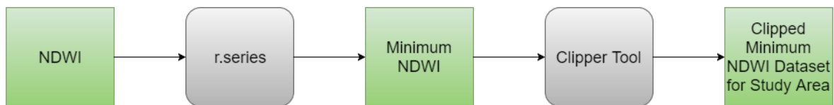
Figure 23: Process to Create Minimum NDWI Dataset.
