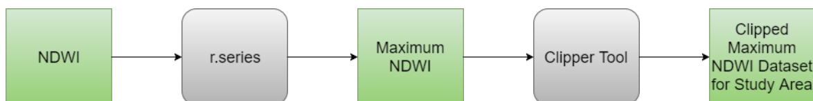
Figure 22: Process to Create Maximum NDWI Dataset.
