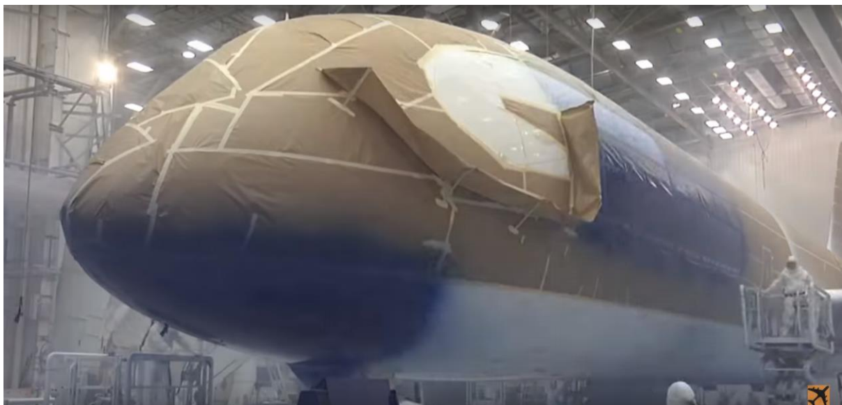
Figure 37: picture of the 777 being painted ( https://www.youtube.com/watch?v=H_olh7qxCbQ )
