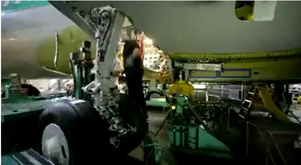
Figure 35: picture of the landing gear being fitted ( https://www.youtube.com/watch?v=H_olh7qxCbQ ).
