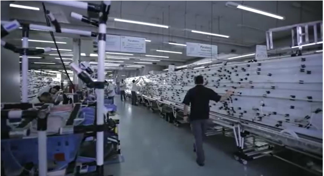
Figure 10: Picture of wiring harnesses being prepared for installation ( https://www.youtube.com/watch?v=XmEuQk5otcg ).
