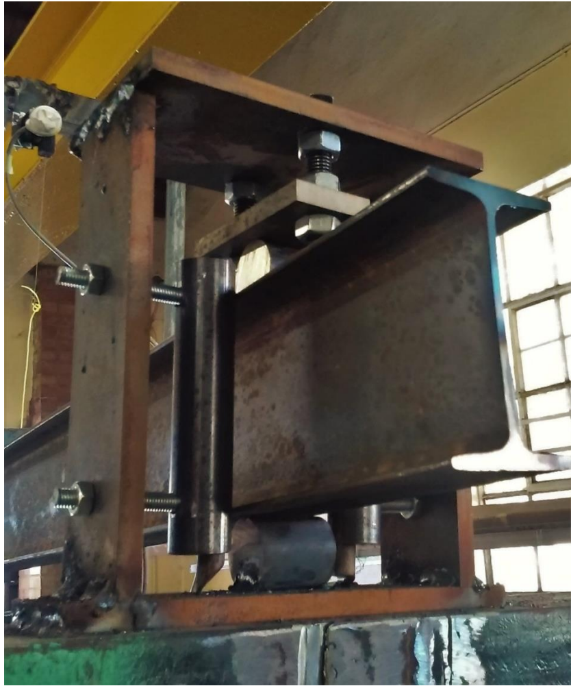
Figure 4.21: Exterior support on top of the existing frame.
