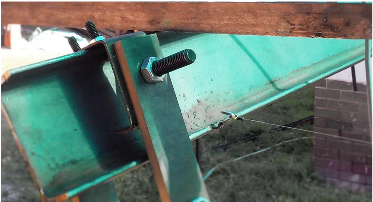
Figure 4.10: String LVDT end attached to a hook to measure displacement.
