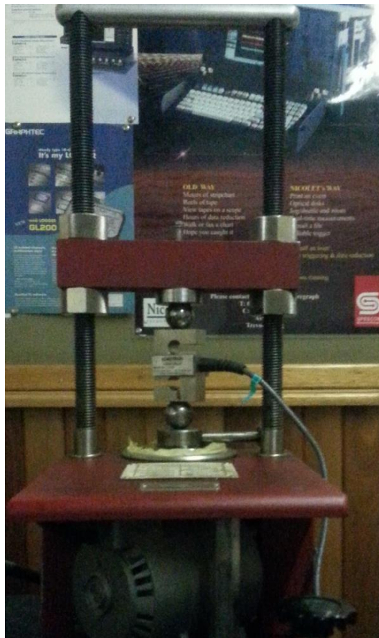
Figure 4.12: Budenberg dead-weight system to calibrate the load cell.
