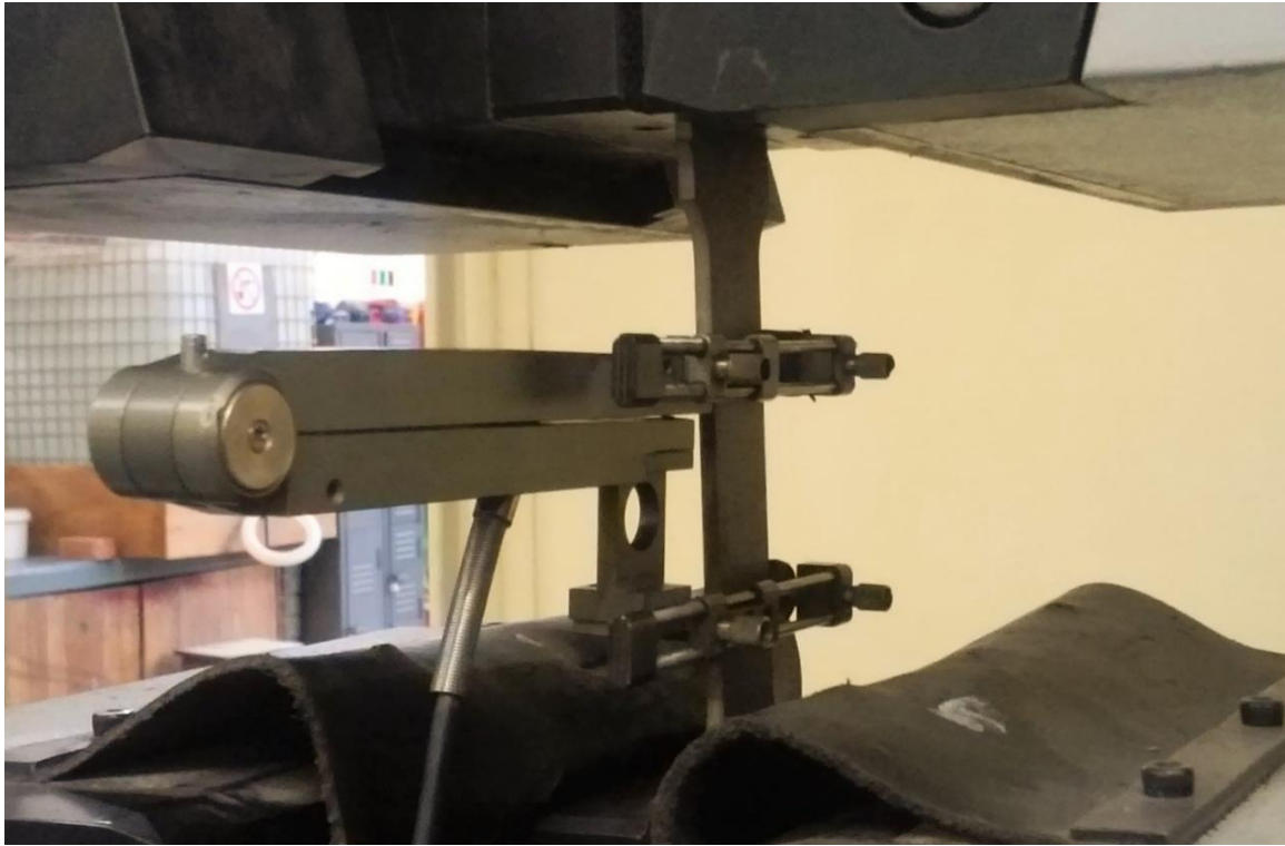
Figure 5.4: Position of clip gauge before testing.
