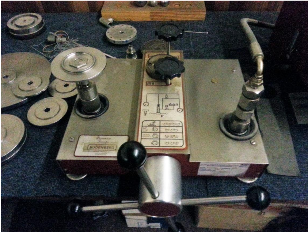
Figure 4.13: Budenberg dead-weight tester that converts the weights to pressure.
