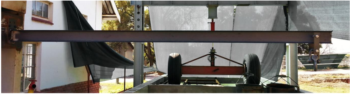
Figure 4.19: Cantilever with shear centre loading (side view).
