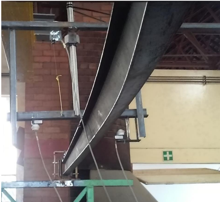
Figure 5.27: Twist in the backspan segment during the experiment.
