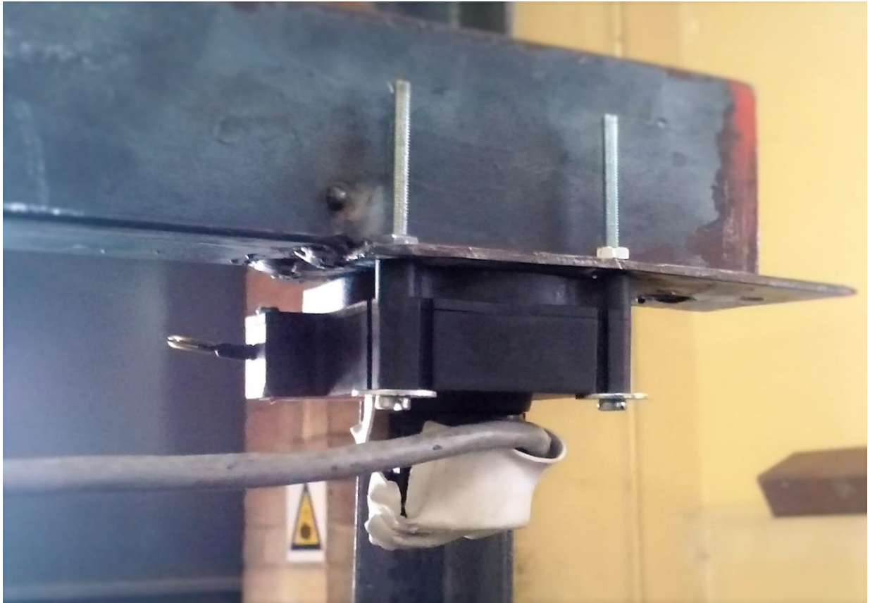
Figure 4.9: A String LVDT that is measuring in the horizontal direction.
