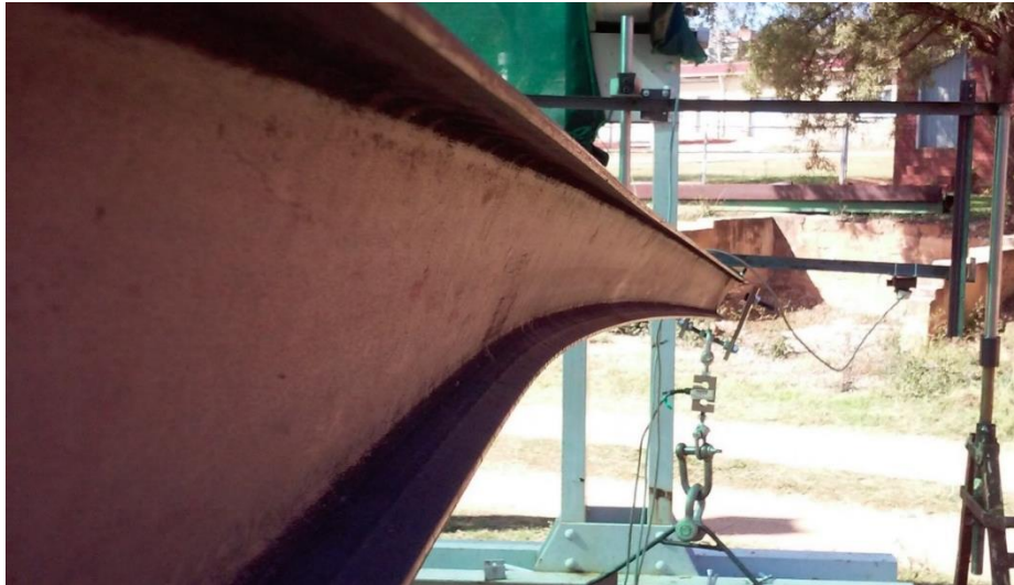
Figure 5.35: Twist of the cantilever during an experiment.
