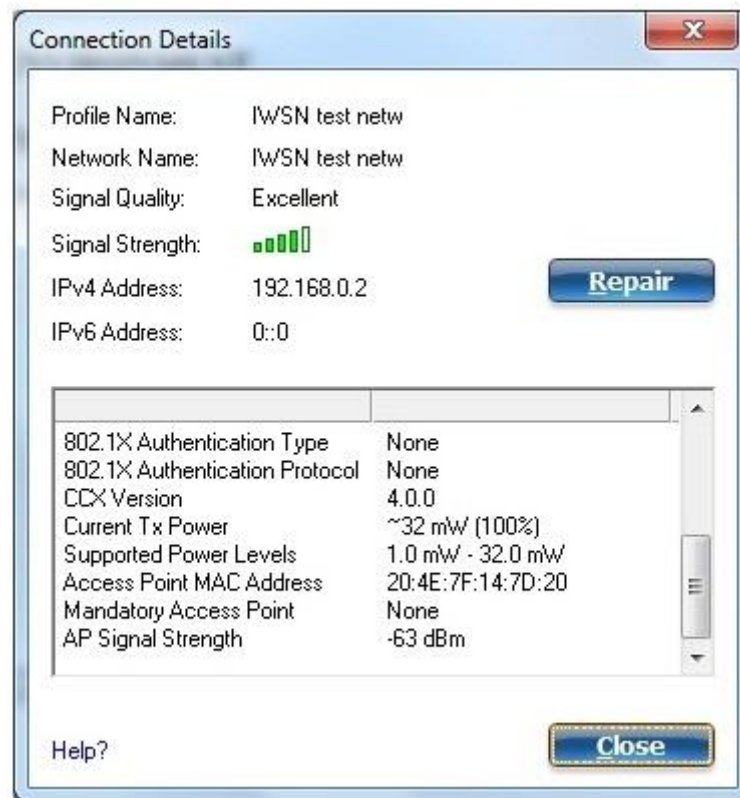
Figure 3.20. Test network extended connection details. Screengrab from Intel's ProSet/Wireless free software.
