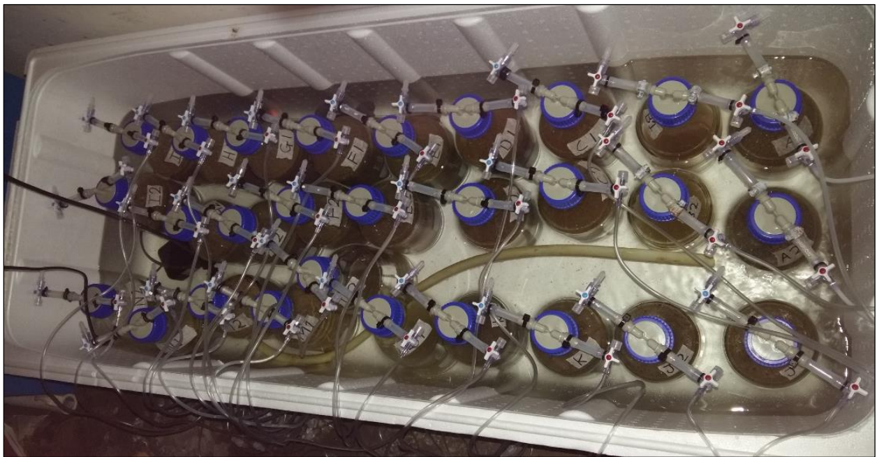
Figure 46: Water bath containing all 28 digester bottles
