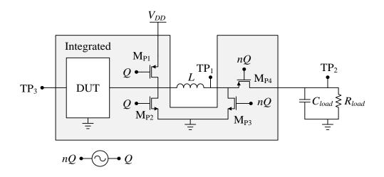
Figure 4.16. Test setup for measuring SenseFET characteristics.
