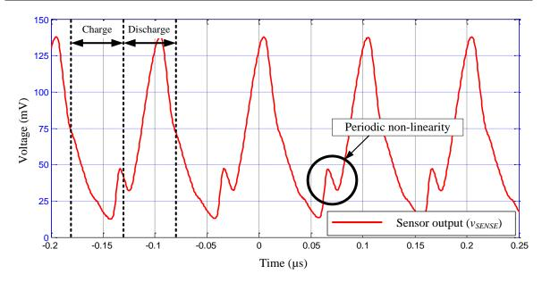
Figure 5.6. Annotated plot of *v*<sub>SENSE</sub> for the cascoded SenseFET.
