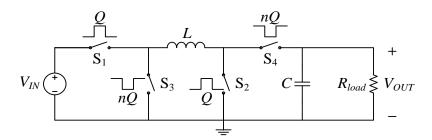
Figure 2.4. Non-inverting DC-DC converter topology.
