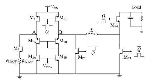
Figure 4.4. SenseFET implemented with a greatly simplified amplifier.
