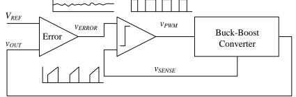
Figure 2.3. Voltage mode control and current mode control topologies.
