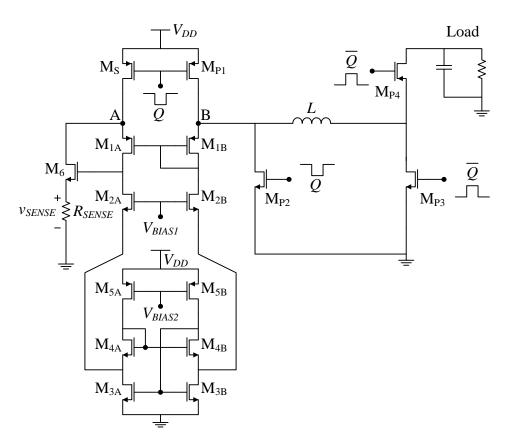
Figure 4.10. Schematic diagram of a SenseFET that has been linearised using a cascode structure.
