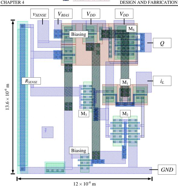
Figure 4.5. CAD Layout of the reference SenseFET.
