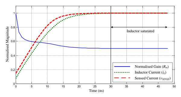
Figure 5.10. Transresistance gain  $(R_m)$ , normalised inductor current, and sensed current of the cascoded SenseFET.
