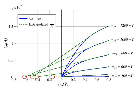
**Figure 4.3.** PFET  $i_{DS} - v_{DS}$  characteristic curves for W/L = 6.
