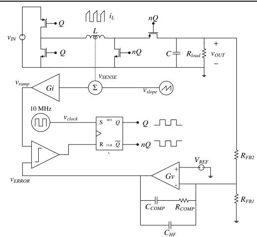
Figure 2.5. Generalised non-inverting buck-boost converter with analogue current mode control.
