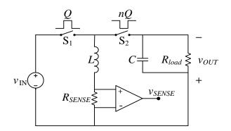
Figure 2.6. Rudimentary current sensing network.
