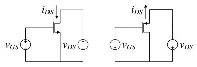
Figure 4.1. Channel length modulation characterisation circuit.
