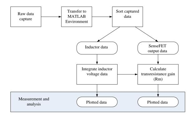
Figure 5.3. Flow diagram describing processing of captured data.
