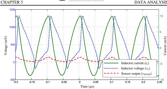
Figure 5.5. Unprocessed data captured from the cascoded SenseFET.
