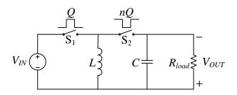
Figure 2.1. Buck-boost voltage converter topology.
