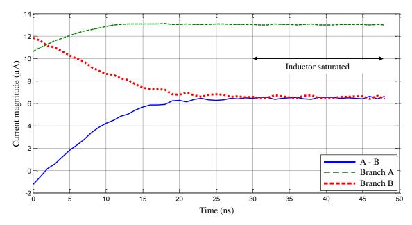
Figure 4.13. Branch currents in cascoded SenseFET.
