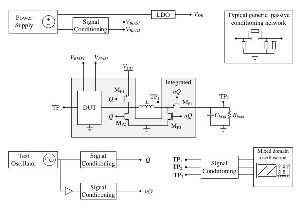
Figure 4.17. Simplified overview of the external test circuit.
