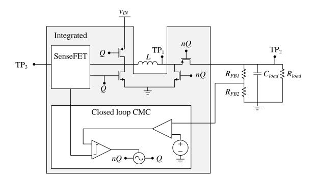
Figure 3.5. Test setup for measuring buck-boost converter.
