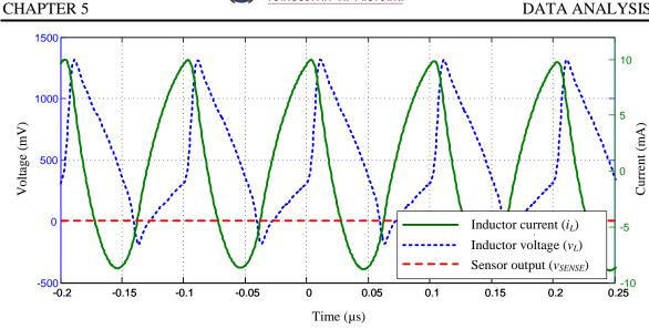
Figure 5.4. Unprocessed data captured from the reference SenseFET.
