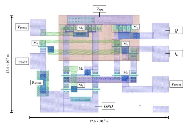
Figure 4.12. CAD Layout of the Cascoded SenseFET.
