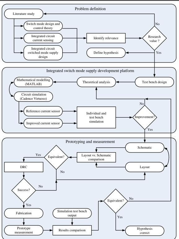
Figure 3.1. Research methodology flow diagram.
