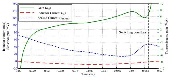
**Figure 5.11.** Cascoded SenseFET gain  $(R_m)$  during inductor discharge.
