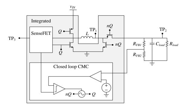
Figure 5.2. Test setup for measuring CMC buck-boost converter performance.
