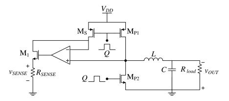
Figure 2.10. Simple SenseFET implemented with idealised components.
