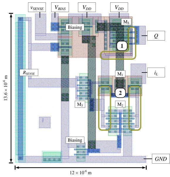
Figure 5.9. Layout of the reference SenseFET with potential layout issues indicated.
