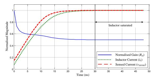
Figure 4.14. Transresistance gain  $(R_m)$ , normalized inductor current, and sensed current of the cascoded SenseFET.
