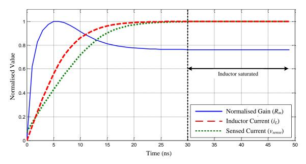
Figure 4.9. Transresistance gain, normalised inductor current, and sensed current of the reference SenseFET.
