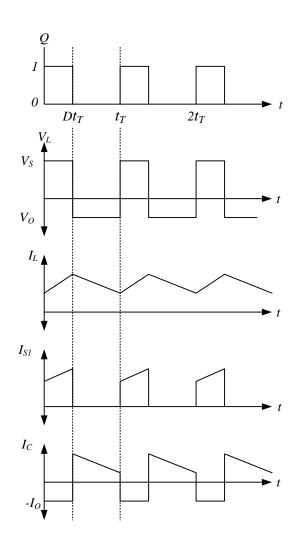
Figure 2.2. Buck-boost converter waveforms.
