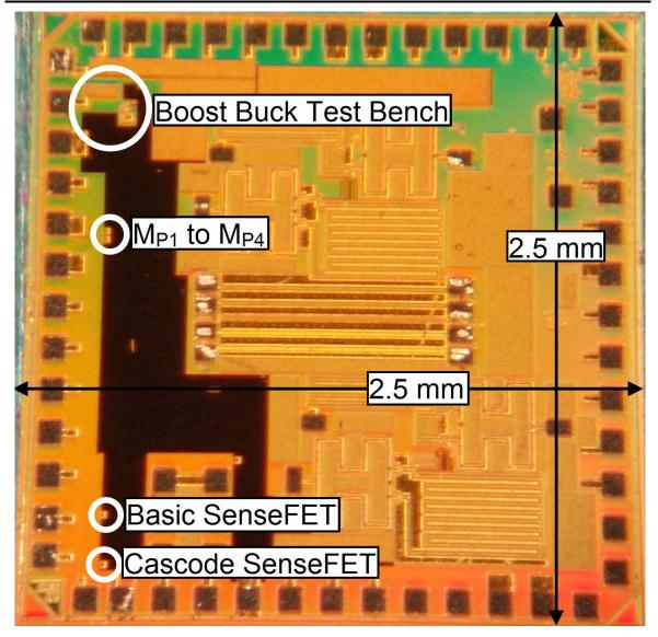
Figure 4.15. Annotated photograph of the manufactured die.
