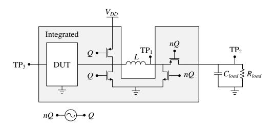
Figure 3.4. Test setup for measuring SenseFET characteristics.
