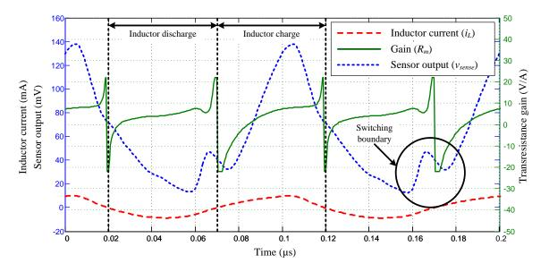
Figure 5.7. Cascode SenseFET performance over a complete switching cycle.
