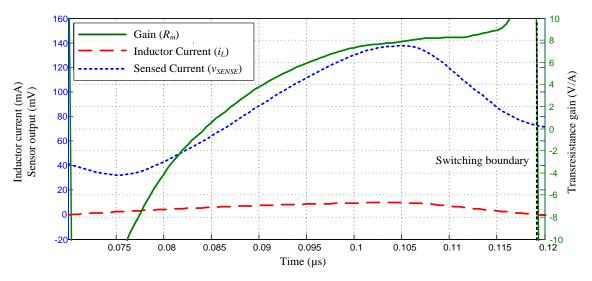
**Figure 5.12.** Cascoded SenseFET gain  $(R_m)$  during inductor charge.
