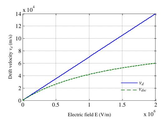
Figure 2.15. Electron drift velocity for linear and approximate models.
