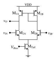
Figure 2.14. Simple CMOS differential amplifier with active load.
