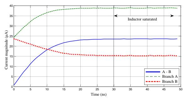
Figure 4.8. Branch currents in reference SenseFET.
