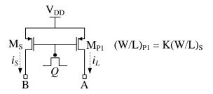
Figure 2.9. Fundamental SenseFET circuit.
