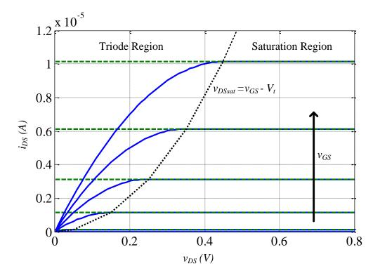
Figure 2.12. Idealised *i*<sub>DS</sub>-*v*<sub>DS</sub> characteristic curves.
