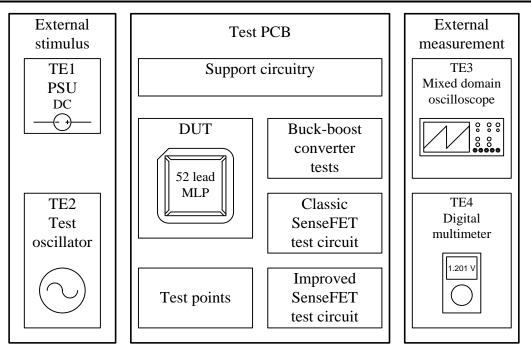
Figure 3.3. Simplified diagram of the test setup and test equipment.
