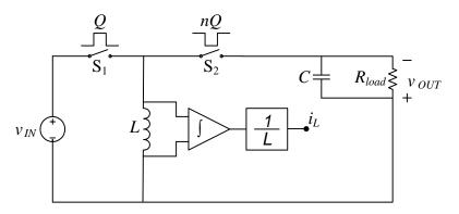
Figure 2.8. Sensorless current sensing circuit.
