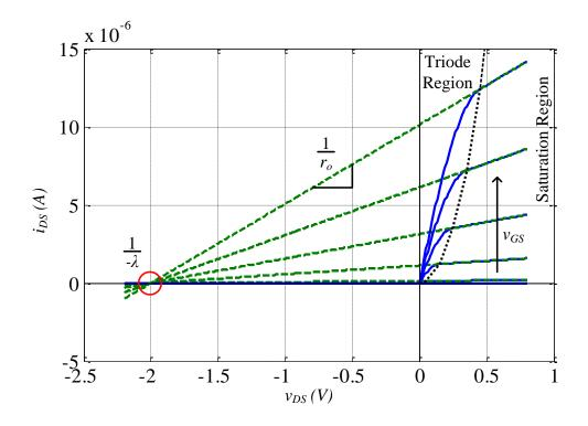
Figure 2.13. *i*<sub>DS</sub>-*v*<sub>DS</sub> characteristic curves with channel length modulation incorporated.
