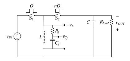
Figure 2.7. Voltage filtering network in shunt with converter inductor.
