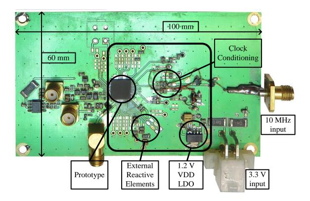
Figure 4.18. Photograph with dimensions of the PCB used to test the prototype IC.
