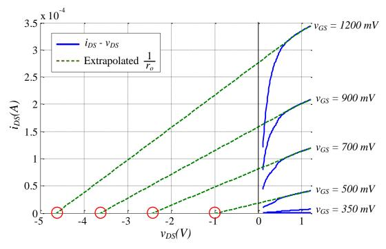
**Figure 4.2.** NFET  $i_{DS} - v_{DS}$  characteristic curves for W/L = 6.
