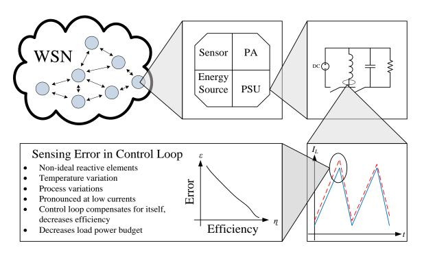
Figure 1.1. Unstructured WSN node requirement breakdown.
