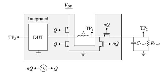
Figure 5.1. Test setup for measuring reference and cascode SenseFETs.
