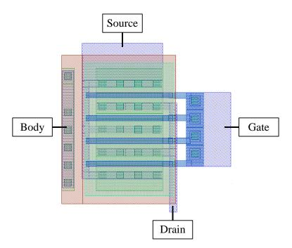
Figure 4.6. PFET Transistor with a fingered gate implementation.
