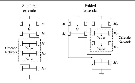
Figure 4.11. Topological difference between standard and folded cascode configurations.
