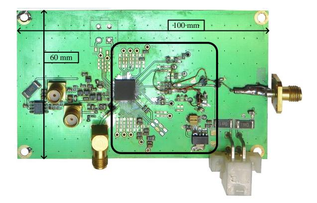
Figure 3.2. Photograph with dimensions of the PCB used to test the prototype IC.
