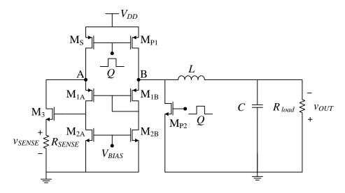
Figure 2.11. SenseFET implemented with a greatly simplified amplifier.
