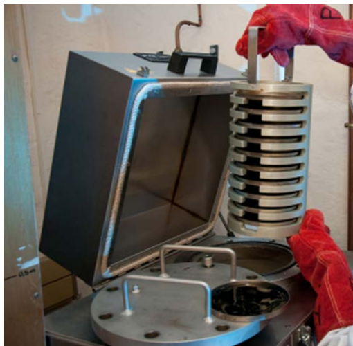
Figure 4: The PAV Ageing Oven at the CSIR.
